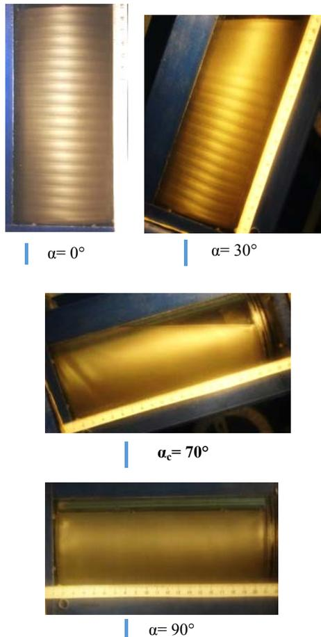
**Fig. 4. Effect of inclination on Taylor vortex flow at  $Ta_1=44\pm 2$  for partially filled system ( $\Gamma = 37$ ). Destruction of Taylor vortices and relaminarization of the flow at  $\alpha_c = 70^\circ$ .**
