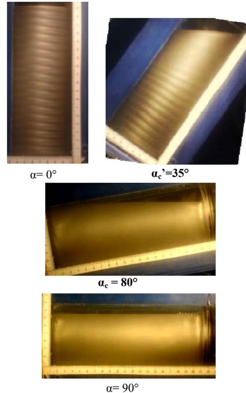
**Fig. 5. Effect of inclination on the wavy vortex flow at  $Ta=56\pm 3$  for partially filled system ( $\Gamma = 37$ ). Disappearance of Wavy mode at  $\alpha_c'=35^\circ$  and flow relaminarization at  $\alpha_c = 80^\circ$ .**
