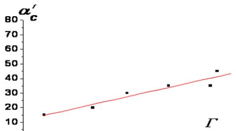
Fig. 7. Critical angle inclination angles  $\alpha'_c$  of the disappearance of WVF versus  $\Gamma$  at  $Ta_{c2} = 56 \pm 3$ .
