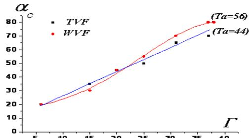
Fig. 6. Critical inclination angles of the relaminarization  $\alpha_c$  versus  $\Gamma$ .
