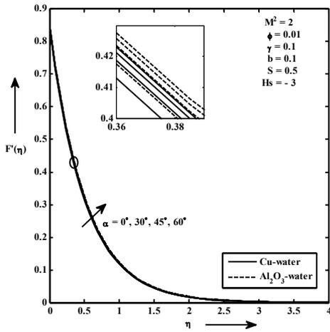
**Fig. 4. Dimensionless velocity profiles for different  $\alpha$**
