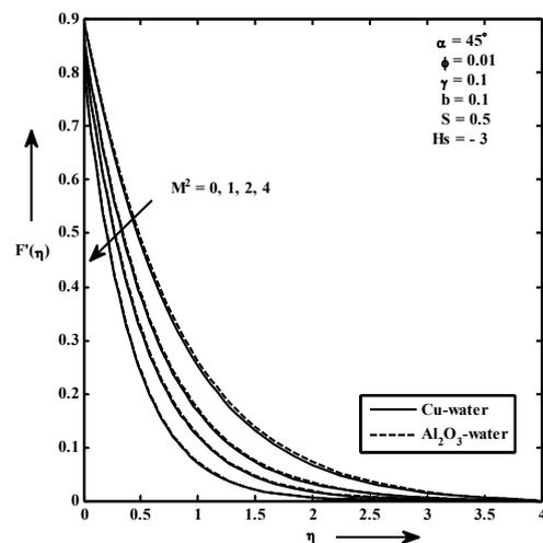
**Fig. 2. Dimensionless Velocity profiles for different  $M^2$ .**
