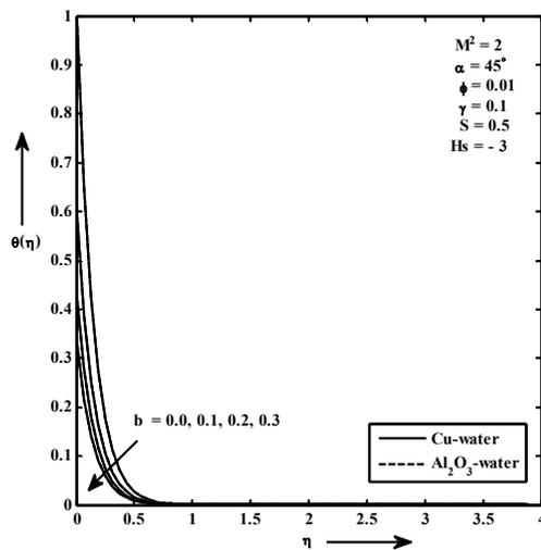
Fig. 9. Temperature distribution for different  $b$ .
