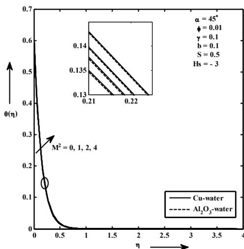
**Fig. 3. Temperature distribution for different  $M^2$ .**
