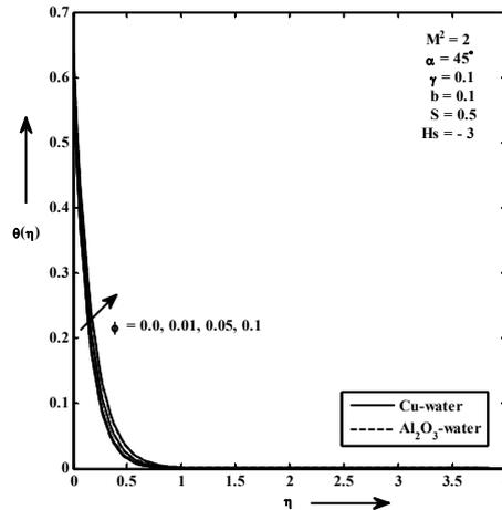
Fig. 7. Temperature distribution for different  $\phi$ .
