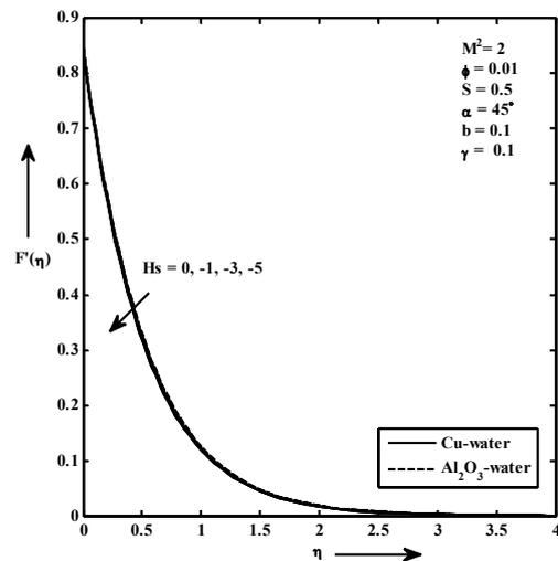
Fig. 12. Dimensionless velocity profiles for different  $H_s$ .
