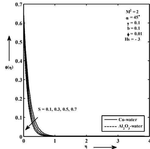
Fig. 11. Temperature distribution for different  $S$ .
