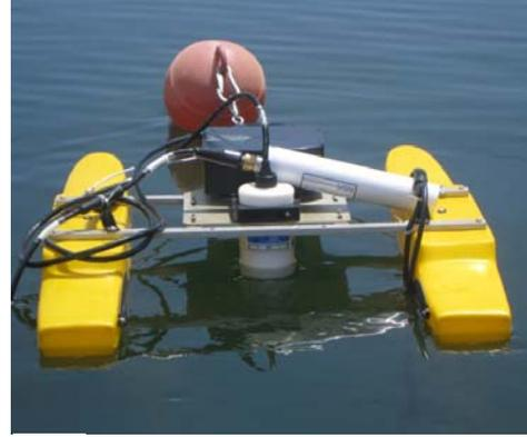
Fig. 3. ADCP and thermistor chain mounted to a buoy to monitor synchronized velocity and temperature data.
