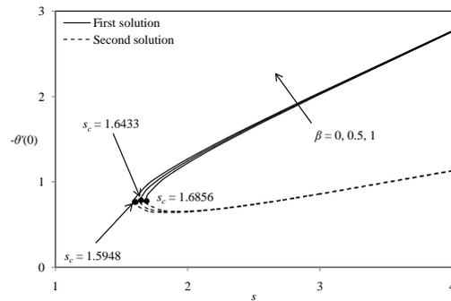
**Fig. 7. Variation of  $-\theta'(0)$  with  $s$  for different  $\beta$  when  $\alpha = 1, Pr = 0.7, \lambda = -1$ .**
