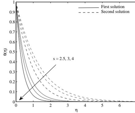
**Fig. 13.** Temperature profiles  $\theta(\eta)$  for different values of  $s$  when  $\alpha = 1, \beta = 0.5, \lambda = -1, Pr = 0.7$ .
