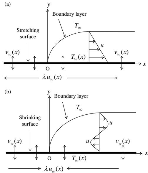
**Fig. 1. The geometry of the problem; (a) stretching surface and (b) shrinking surface.**
