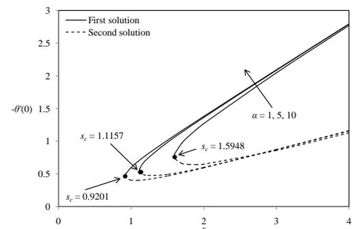
**Fig. 11. Variation of  $-\theta'(0)$  with  $s$  for different  $\alpha$  when  $\beta = 1, Pr = 0.7, \lambda = -1$ .**
