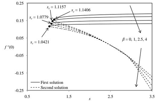
**Fig. 8. Variation of  $f''(0)$  with  $s$  for different  $\beta$  when  $\alpha = 5, Pr = 0.7, \lambda = -1$ .**
