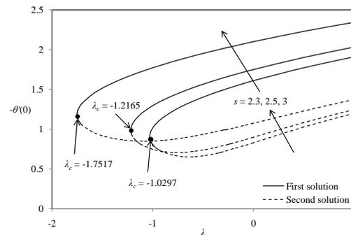
**Fig. 5.** Variation of  $-\theta'(0)$  with  $\lambda$  for different  $s$  when  $Pr = 0.7$ ,  $\alpha = \beta = 0$  (no slip).
