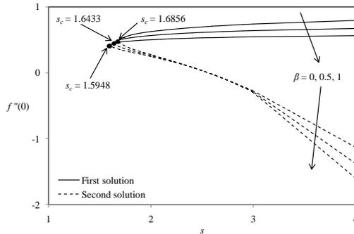
**Fig. 6. Variation of  $f''(0)$  with  $s$  for different  $\beta$  when  $\alpha = 1, Pr = 0.7, \lambda = -1$ .**
