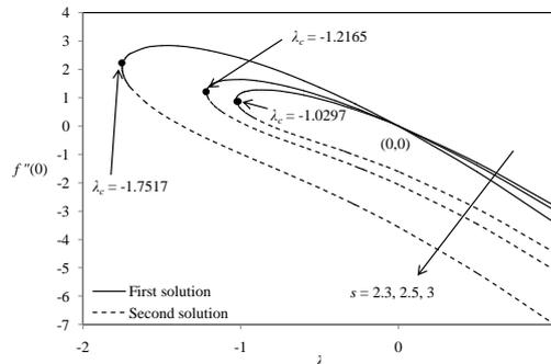
**Fig. 4.** Variation of  $f''(0)$  with  $\lambda$  for different  $s$  when  $Pr = 0.7$ ,  $\alpha = \beta = 0$  (no slip).
