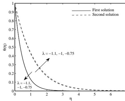
**Fig. 15.** Temperature profiles  $\theta(\eta)$  for different values of  $\lambda$  when  $\alpha = 1, \beta = 0.5, s = 3, Pr = 0.7$ .
