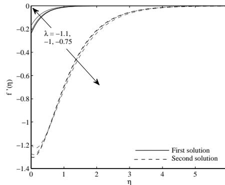
**Fig. 14.** Velocity profiles  $f'(\eta)$  for different values of  $\lambda$  when  $\alpha = 1, \beta = 0.5, s = 3, Pr = 0.7$ .
