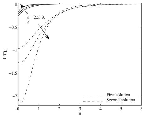
**Fig. 12.** Velocity profiles  $f'(\eta)$  for different values of  $s$  when  $\alpha = 1, \beta = 0.5, \lambda = -1, Pr = 0.7$ .
