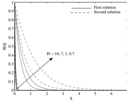
**Fig. 16. Temperature profiles  $\theta(\eta)$  for different values of  $Pr$  when  $\alpha = 1$ ,  $\beta = 0.5$ ,  $s = 3$ ,  $\lambda = -1$**
