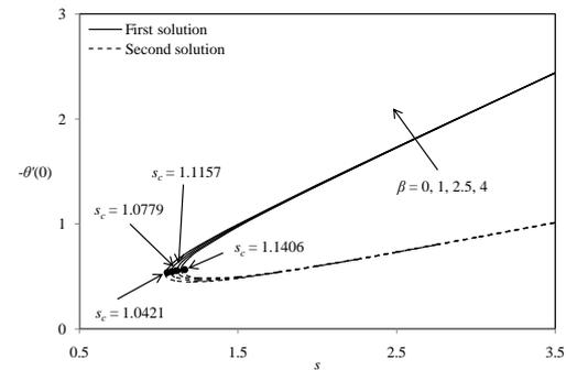
**Fig. 9. Variation of  $-\theta'(0)$  with  $s$  for different  $\beta$  when  $\alpha = 5, Pr = 0.7, \lambda = -1$ .**
