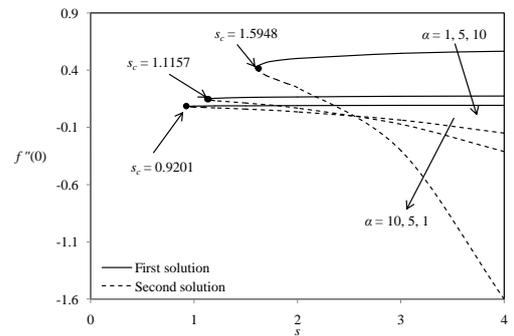
**Fig. 10. Variation of  $f''(0)$  with  $s$  for different  $\alpha$  when  $\beta = 1, Pr = 0.7, \lambda = -1$ .**
