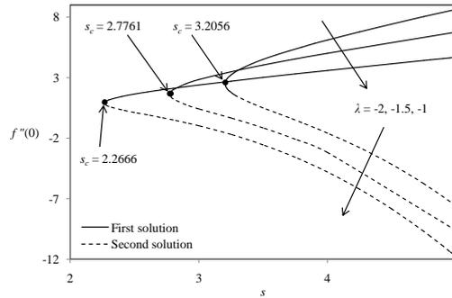
**Fig. 2.** Variation of  $f''(0)$  with  $s$  for different  $\lambda$  when  $Pr = 0.7$ ,  $\alpha = \beta = 0$  (no slip).
