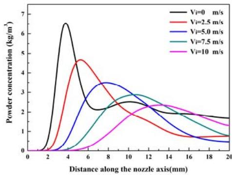
**Fig. 9. Powder concentration along the nozzle axis with various inner shielding gas rate when carrier gas rate is 1m/s, outer shielding gas rate is 5m/s, and powder feed rate is 4.1g/min.**
