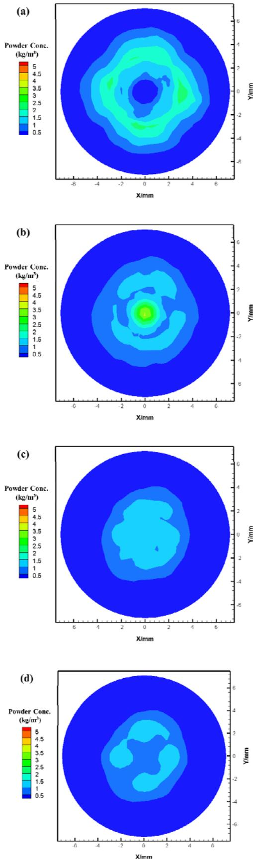
**Fig. 7. Powder concentration distribution in transverse section with nozzle exit displacement of (a) 2.5 mm, (b) 8 mm, (c) 15 mm, and (d) 18 mm.**
