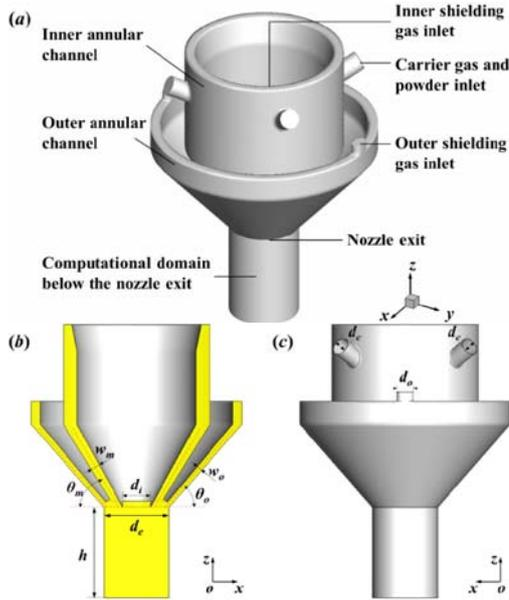
**Fig. 2.** The geometry model of the computational domain. (a) isometric view; (b) sectional view; (c) back view.
