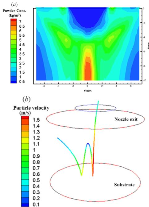
**Fig. 13. The effect of flat substrate on the powder flow: (a) the powder concentration distribution below the coaxial nozzle; (b) rebound of a particle on the substrate.**
