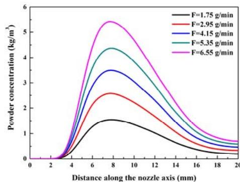
**Fig. 12. Powder concentration along the nozzle axis with various powder feed rate when inner shielding gas rate is 5m/s, carrier gas rate is 1m/s, and outer shielding gas rate is 5m/s.**
