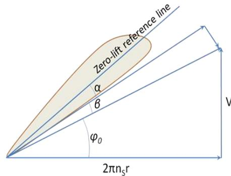
**Fig. 6. Diagram of blade element and airflow.**
