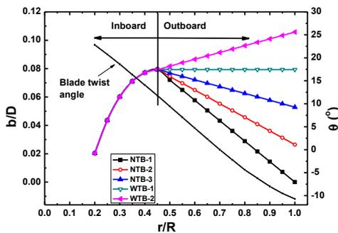
c) Geometric parameters along radius
