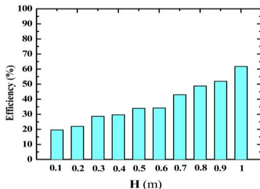
**Fig. 5.** Duct efficiency for different duct height.
