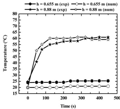
**Fig. 2. The temperature distribution measured in the corridor: Curve Validation.**
