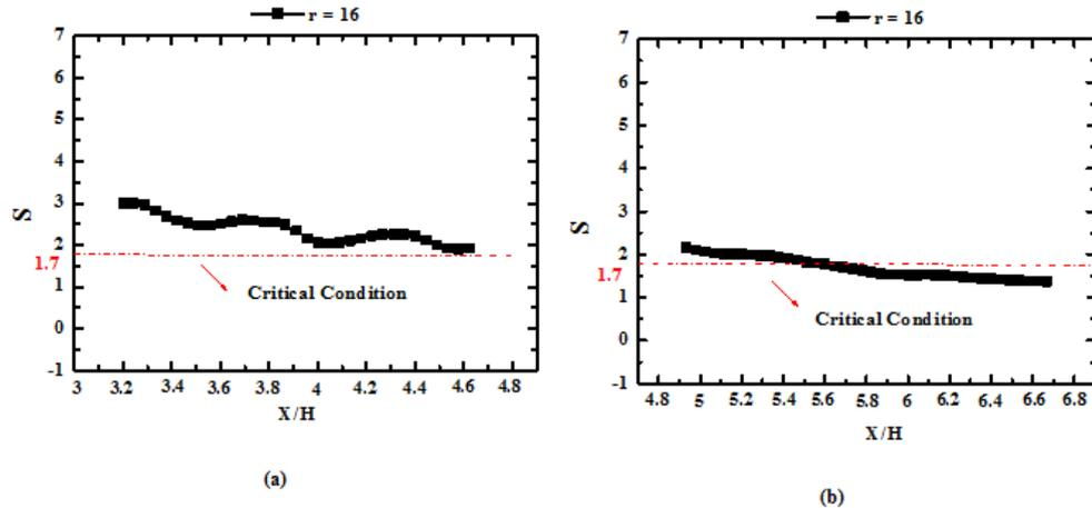
**Fig. 11. The longitudinal evaluation of the stratification parameter (based on Newman, 1984) for  $r = 16$ : (a) the upstream view, (b) the downstream view.**
