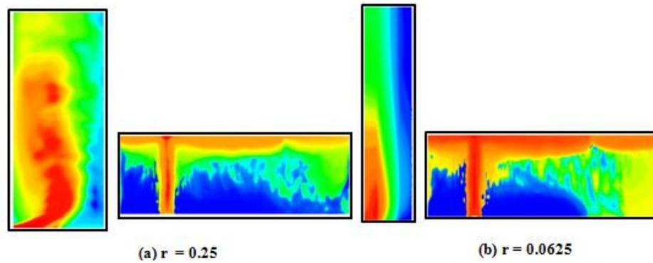
Fig. 8 Temperature contour distribution with various duct shape in the corridor and in the duct.
