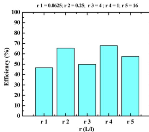
**Fig. 7. Duct efficiency as a function of different aspect ratio (r): Variation of the duct shape.**
