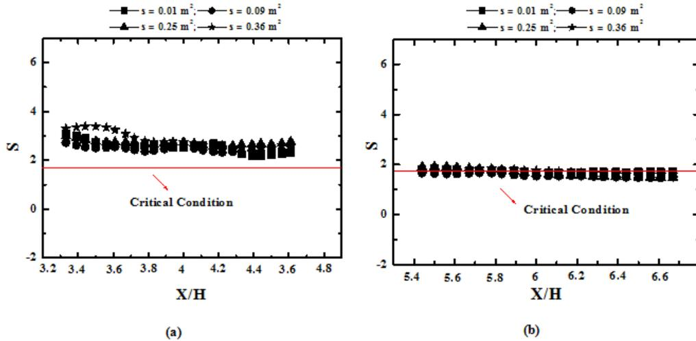
Fig. 9. The longitudinal evaluation of the stratification parameter (based on Newman, 1984) with the duct section variation: (a) the upstream view, (b) the downstream view.
