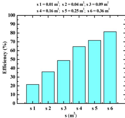
Fig. 3. Duct efficiency for different duct section.
