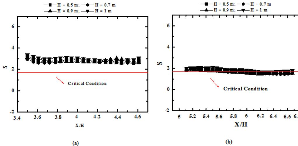
Fig. 10. The longitudinal evaluation of the stratification parameter (based on Newman, 1984) with the duct height variation: (a) the upstream view, (b) the downstream view.
