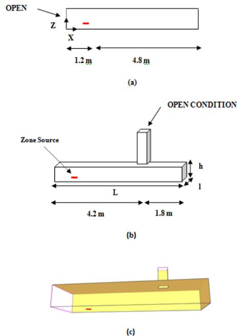
Fig. 1. Schematic 2D (a) and 3D (b) views of the tunnel, and FDS computational model.
