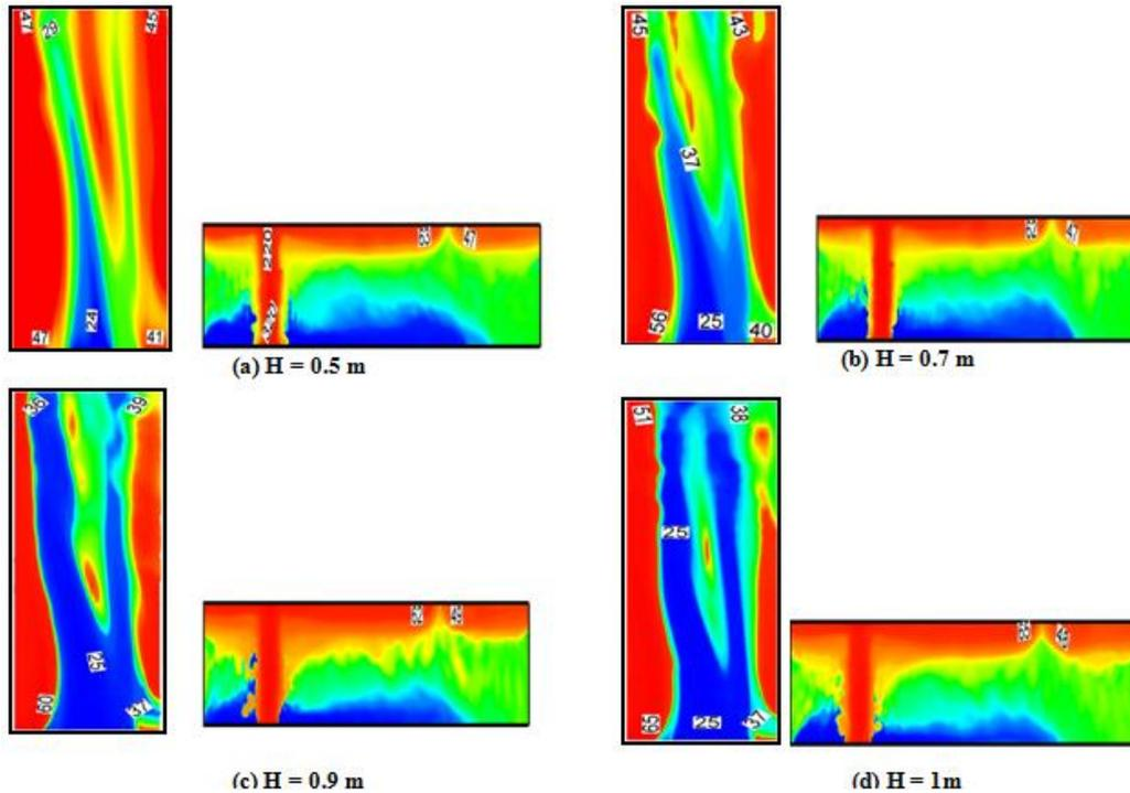
**Fig. 6. Temperature contour distribution with various duct height in the corridor and in the duct (In the left side: duct system; In the right side: the corridor).**
