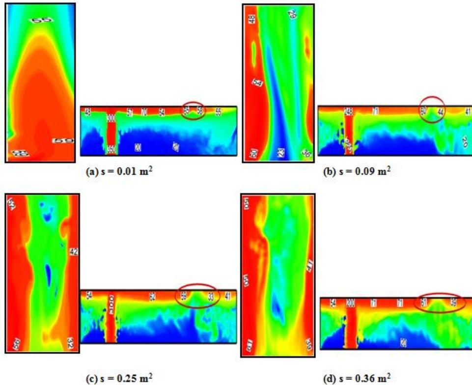
**Fig. 4.** Temperature Contour distribution with various duct section in the corridor (The zone sunken is circulated on red) and in the duct (In the left side: duct system; In the right side: the corridor).
