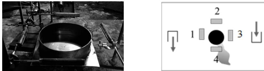
Fig. 8. Picture and schematic diagram of the positions of oxygen analyzers near the fuel pan.
