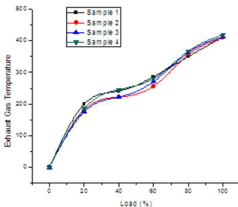
Fig. 5. Exhaust gas temperature vs Load
