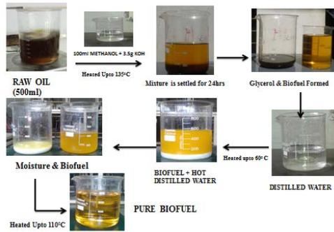
**Fig.1. Transesterification of vegetable oil to biodiesel**
