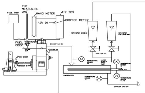
**Fig. 2. Schematic layout of Experimental setup**
