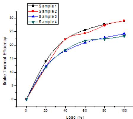
Fig. 4. Brake thermal efficiency vs Load
