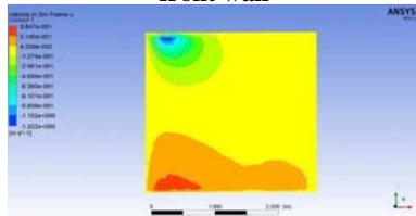
**Fig. 2(c) Velocity distribution at 3feet from the rear wall**
