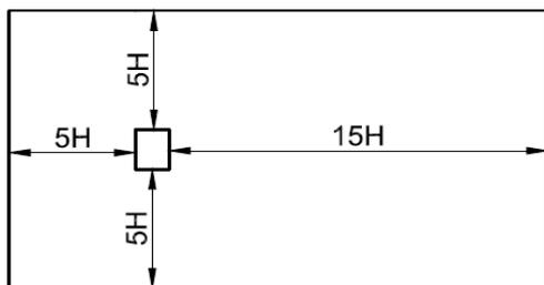
Fig. 1. Position of outlet at the top of the building
