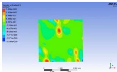
**Fig. 3(a) Velocity distribution at 5feet (Middle of the room)**
