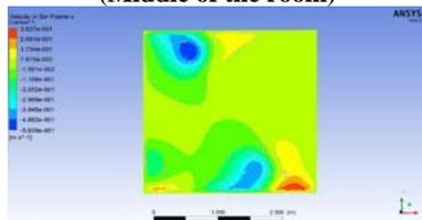
**Fig. 2(b) Velocity distribution at 3feet from the front wall**
