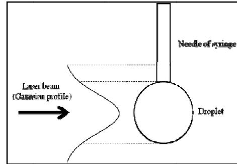
**Fig. 3. Hitting of laser beam to the droplet and the needle.**
