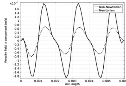
Fig. 6. Second order x-velocity velocity profile at middle height.
