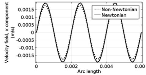
Fig. 5. First order x-velocity velocity profile at middle height.
