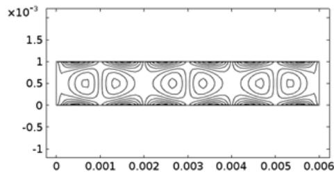
**Fig. 9. Acoustic streaming inner and outer boundary layer for Newtonian viscosity model.**
