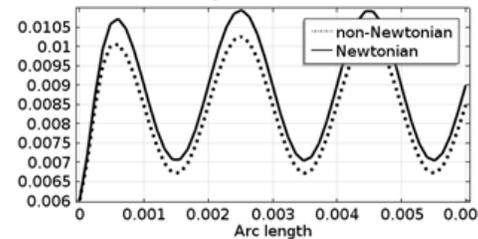
Fig. 7. Total x-velocity profile at middle height.
