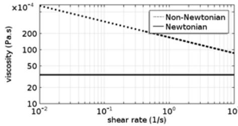
Fig. 2. Viscosity as a function of shear rate.
