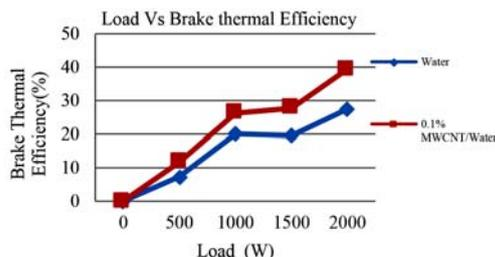
Fig.7 Effect of load on brake thermal efficiency.
