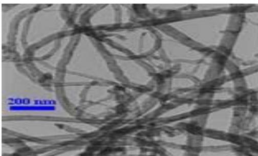
Fig. 1. SEM micrograph of MWCNT.
