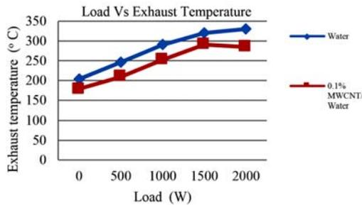
Fig. 5. Effect of load on exhaust temperature.
