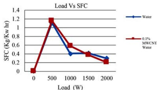
Fig. 6. Effect of load on specific fuel consumption.
