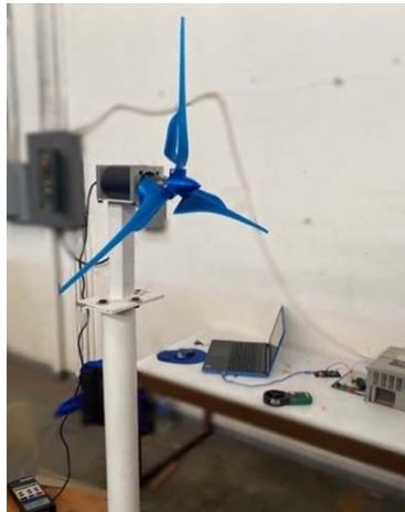
Fig. 9. Bench test of the Induction Blade.
