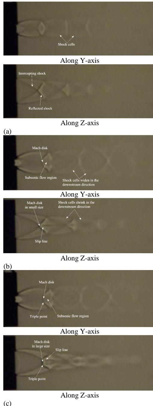
**Fig. 8. Shadowgraph views of the elliptic jet at (a) NPR 3 (b) NPR 4 (c) NPR 5.**
