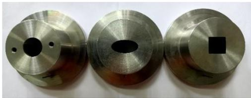
**Fig. 4. Image of the circular, elliptic, and square nozzles.**
