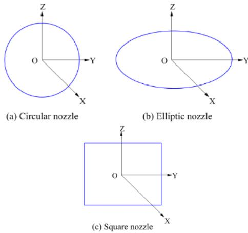
**Fig. 3. Schematic views of the nozzle outlet geometries**
