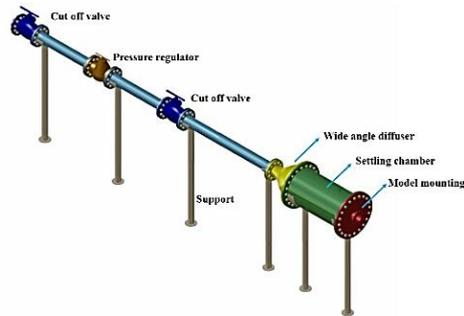
**Fig. 1. Schematic view of the free jet-testing setup.**
