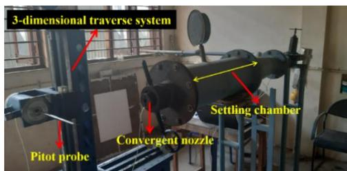
**Fig. 2. Photographic view of the free jet-testing setup.**
