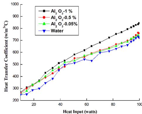
**Fig. 7. Heat Input Vs Heat transfer coefficient.**
