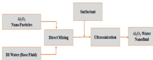
Fig. 2. Two-step method.
