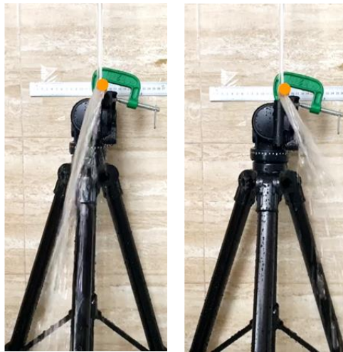
(a) Negative deflection of jet (b) Positive deflection of jet
