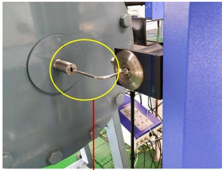
Pitot probe placed at the Nozzle exit
