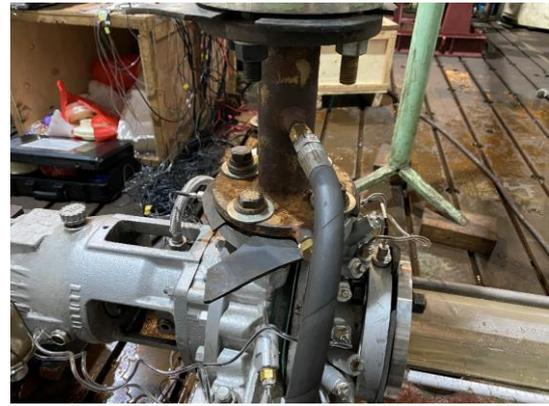
Fig. 1 Single-stage cantilever PAT
