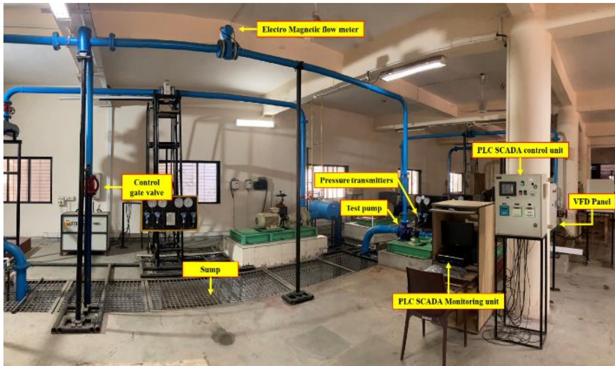
Fig. 13 Actual experimental view of the open loop test bench
