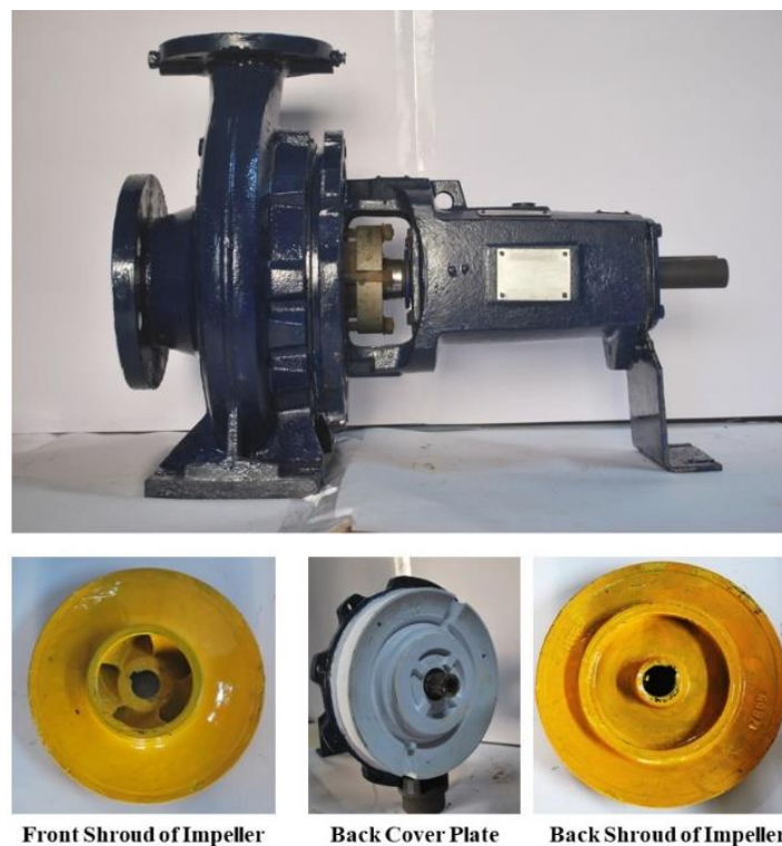
Fig. 5 Geometry of the analyzed centrifugal pump
