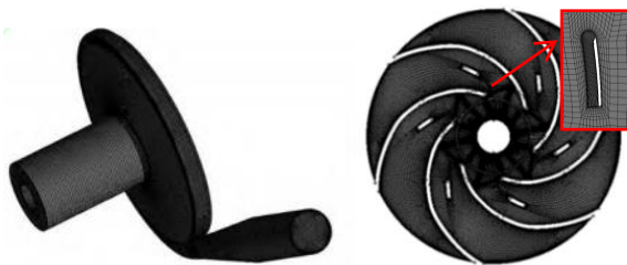
Fig. 3(a) Computational domain meshing for the centrifugal pump
