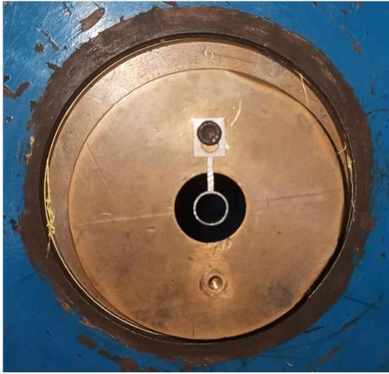
**Fig. 4** Photographic view of the circular ring tab mounted at the nozzle exit
