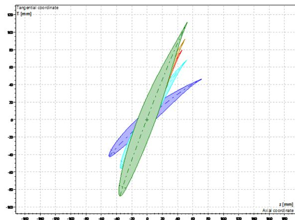
**Fig. 13 Section designs of the optimal fan blade**
