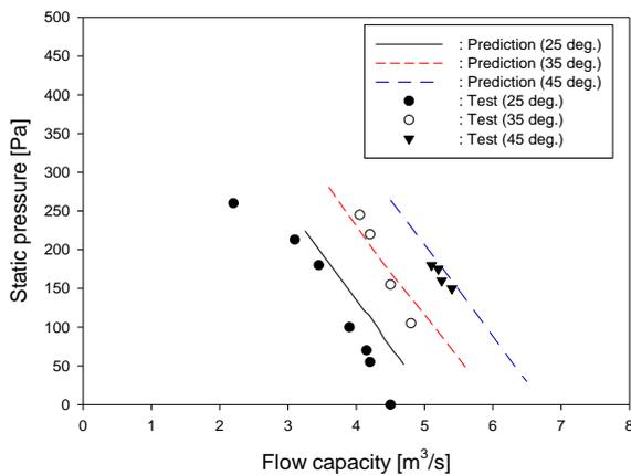
Fig. 6 Pressure curves of axial flow fan
