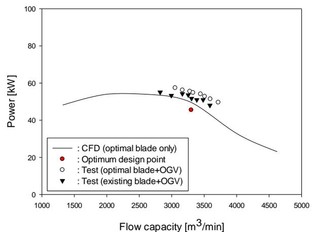
**Fig. 21** Power curve of the optimal fan blade
