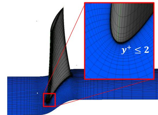
**Fig. 15 Mesh system for the optimal fan blade**
