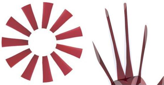
**Fig. 14 3-D shape of the optimal fan blade**
