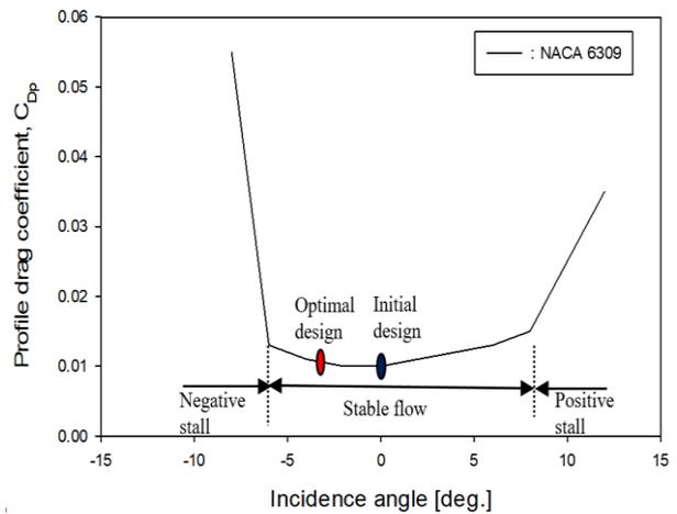
**Fig. 12 Design incidence angle comparison between the optimal and the initial fan designs**
