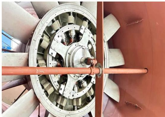
**Fig. 18** Assembly of manufactured optimal fan blades
