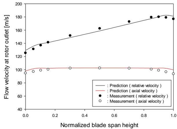
**Fig. 3 Velocity distributions of axial compressor**
