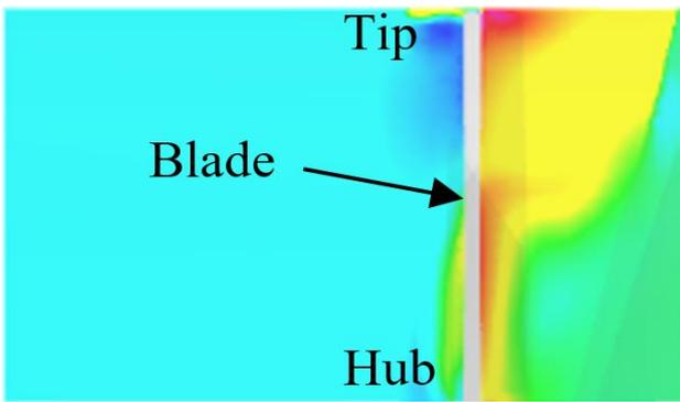
**Fig. 17** Total pressure distribution of air passing through the optimal fan blade
