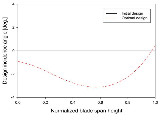
**Fig. 11 Design incidence angle distribution of the optimal fan blade**
