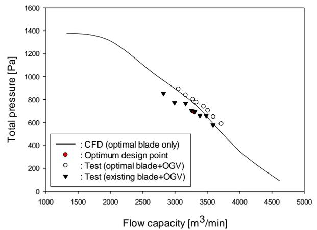
**Fig. 19** Total pressure curve of the optimal fan blade
