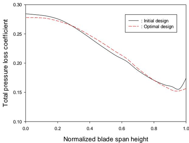
**Fig. 10 Total pressure loss coefficient distribution of the optimal fan blade**
