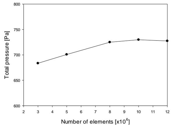
**Fig. 16 Mesh dependency test**
