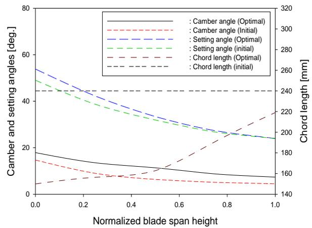
Fig. 9 Camber and setting angle distributions of the optimal fan blade
