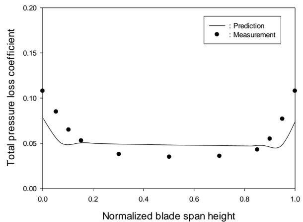
**Fig. 4 Pressure loss distribution of axial compressor**
