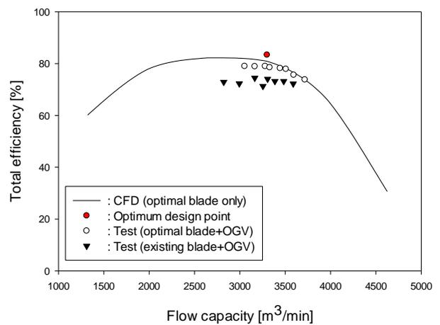
**Fig. 20** Efficiency curve of the optimal fan blade
