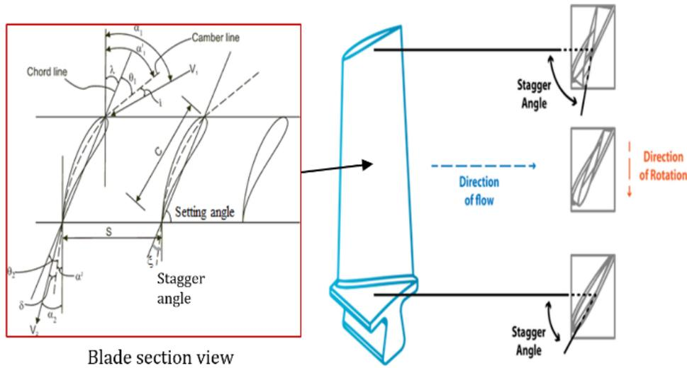
Fig. 1 Fan blade section and design parameters
