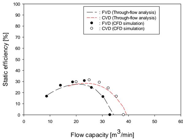
Fig. 5 Efficiency curves of axial flow fans
