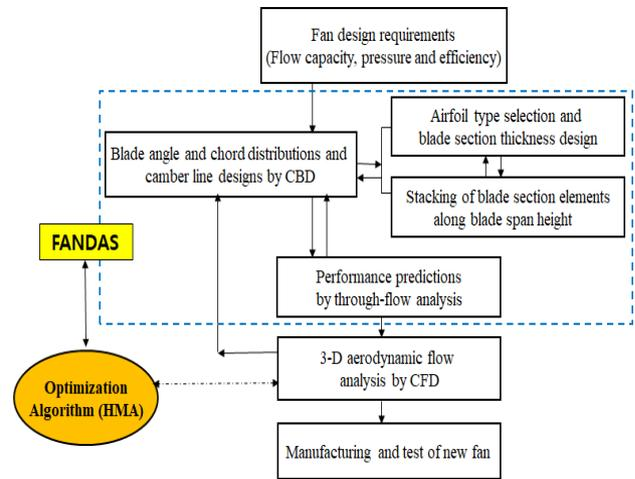
Fig. 2 Computation process of the design and through-flow analysis of axial fan
