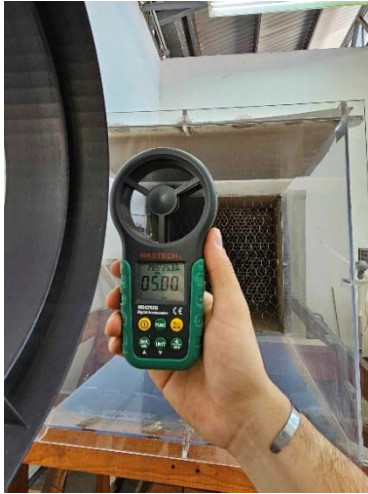
Fig. 13 Measuring of the wind with an anemometer
