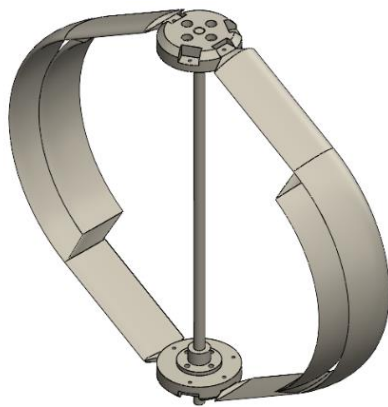
Fig. 11 Isometric view of the assembling the 3D-printed turbine for “Flow concentrator blade”
