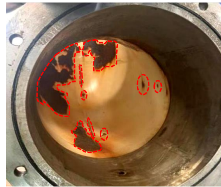
Fig. 11 Damage to the bend section of the draft pipe
