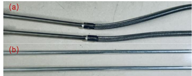
Fig. 3 Diagram of connection pipe: (a) Stainless steel bellows; (b) Aluminum tube
