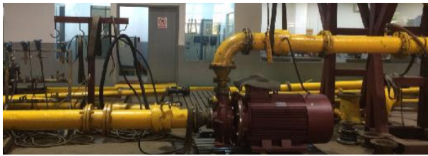
(a) Test section for hydraulic performances of the model fire pump.
