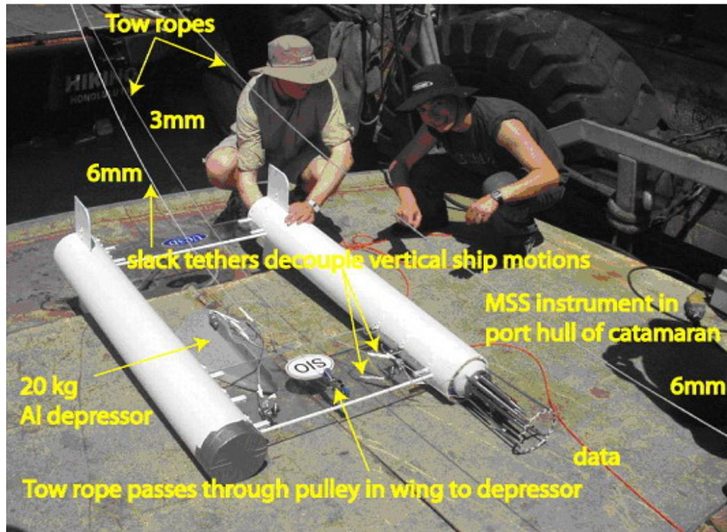
**Fig. 13** - Catamaran tow body with MSS instrument mounted in port hull. Tow speeds of  $2 \text{ m s}^{-1}$  exceeded the maximum speed permitted for shear sensors. Micro-temperature, micro-conductivity, micro-turbidity sensors and mean T, C and P sensors were operational.
