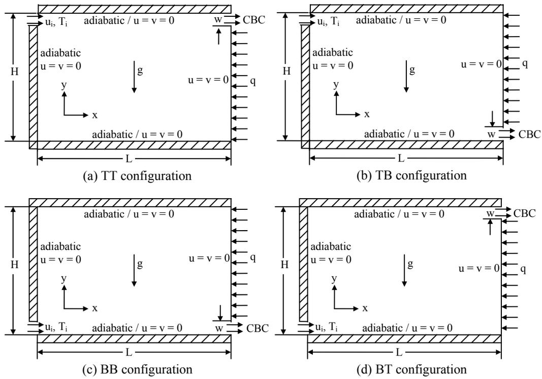
**Fig. 1-** Four schematic configurations of thermally driven cavity
