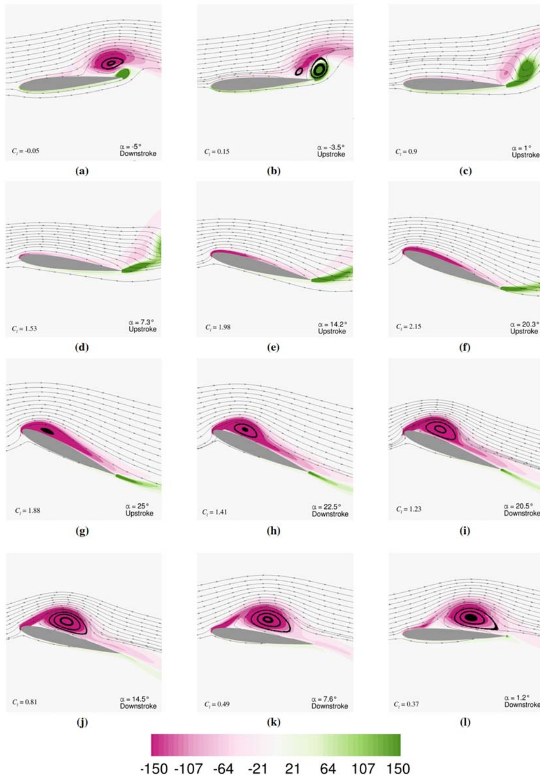
Fig. 9. Development of the leading edge vortex colored by spanwise vorticity value in [1/s].
