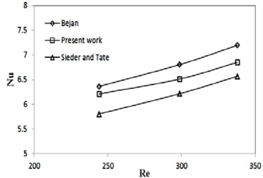
**Fig. 4. Comparison between the experimental results and the theoretical values obtained from the relations of Sieder and Tate (Eq. 18) and Bejan (Eq. 19).**
