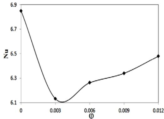
Fig. 6. Variations of Nu with  $\phi$  at constant coolant flow rate of 13lit/min.
