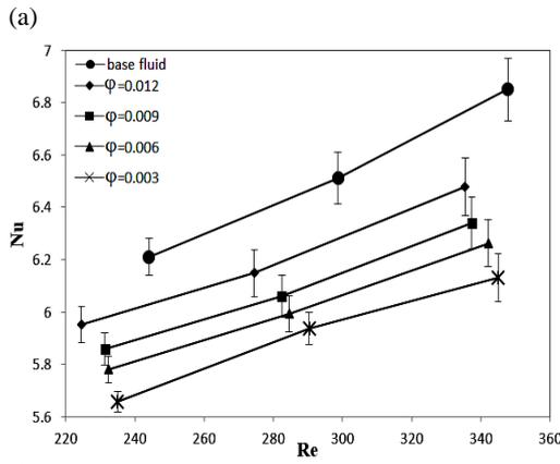
**Fig. 8. Variations of  $Nu$  with a) coolant volumetric flow rate, b)  $Re$  number.**
