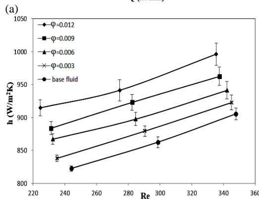
Fig. 7. Variations of h with a) coolant volumetric flow rate, b) Re number.
