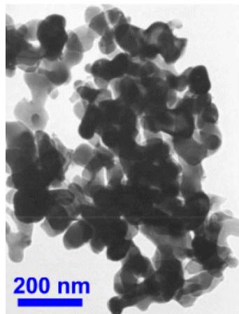
**Fig. 3. TEM image of the Al<sub>2</sub>O<sub>3</sub> nanoparticles.**
