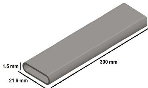
Fig. 2. Schematic and dimensions of the radiator flat tube.
