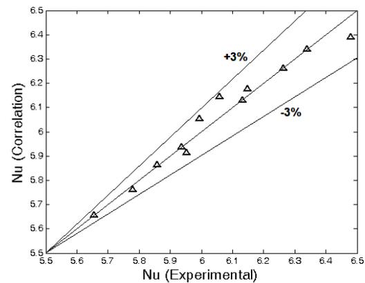
**Fig. 10. Comparison of the correlation and experimental results.**
