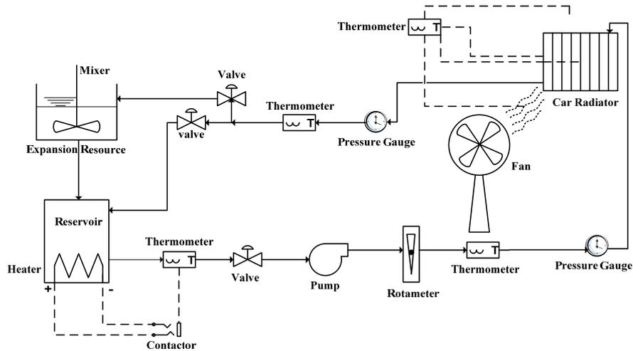
Fig. 1. A schematic diagram of the experimental set up.
