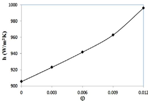
Fig. 5. Variations of convective heat transfer coefficient with  $\phi$  at coolant flow rate of 13 lit/min.
