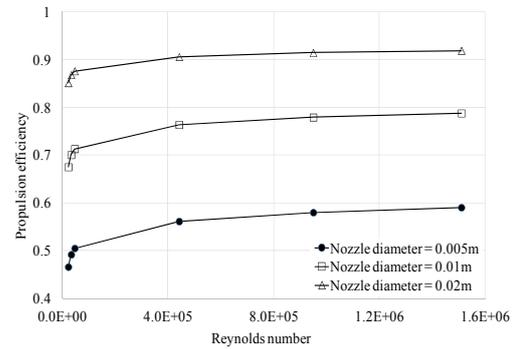
**Fig. 20. Variation of propulsive efficiency with Reynolds number for three different nozzle diameters.**
