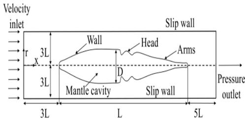
**Fig. 12. Computational domain and boundary conditions of the numerical model.**
