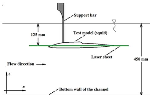
**Fig. 10.** Schematic view of the experimental set-up.
