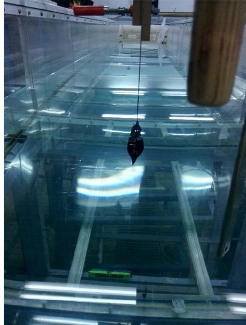
**Fig. 7. Close-circuit water channel and printed squid model.**
