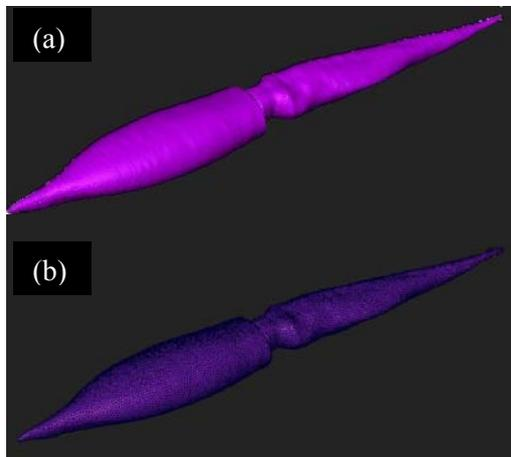
**Fig. 5. Surface model after segmentation (top) surface model after defect cleaning and smoothing (bottom).**
