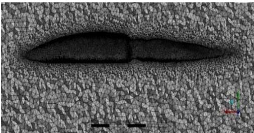
**Fig. 13. Tetrahedral and quadrilateral mesh elements in the solution domain.**
