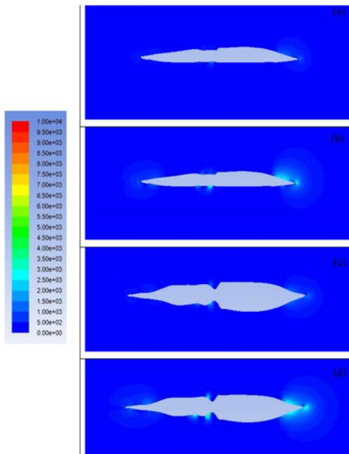
**Fig. 16. Pressure contour plot for Reynolds numbers of 949900 (a, c) and 1510400 (b, d). The front and top views of the squid model were illustrated in (a, b) and (c, d), respectively.**
