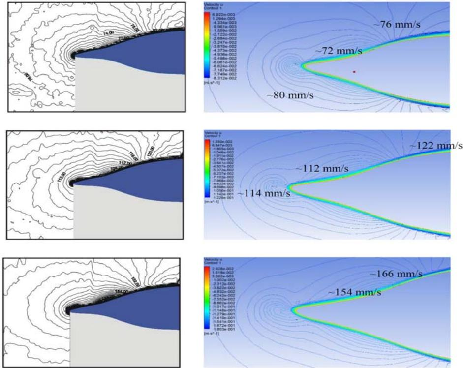
Fig. 14. Comparison of DPIV and CFD velocity contour plots for inlet velocities of 78.6 mm/s (upper), 115.7 mm/s (middle) and 160.1 mm/s (lower).
