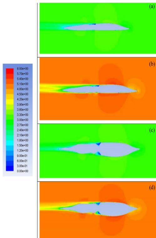
Fig. 15. Velocity contour plot for Reynolds numbers of 949900 (a, c) and 1510400 (b, d). The front and top views of the squid model were illustrated in (a, b) and (c, d), respectively.
