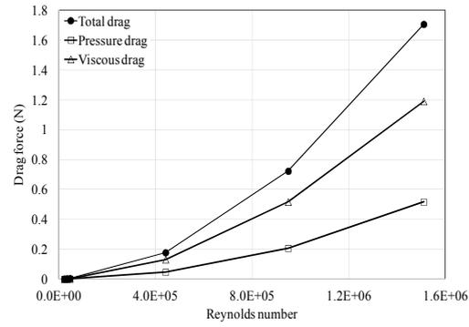
**Fig. 17. Variation of total, pressure and viscous drag along with Reynolds number.**
