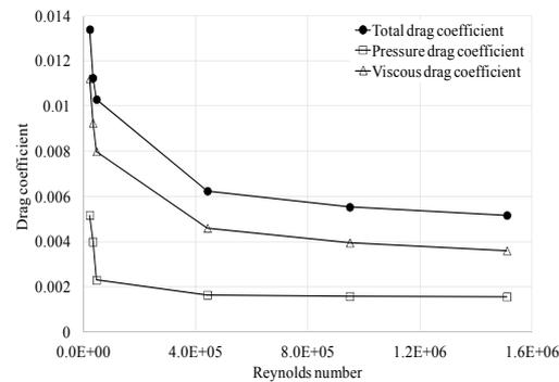
**Fig. 18. Variation of total, pressure and viscous drag coefficient along with Reynolds number.**
