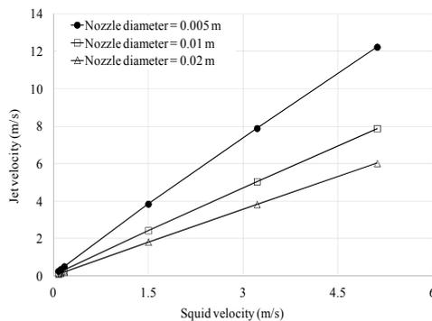
**Fig. 19. Relationship between squid velocity and jet velocity for three different nozzle diameters.**
