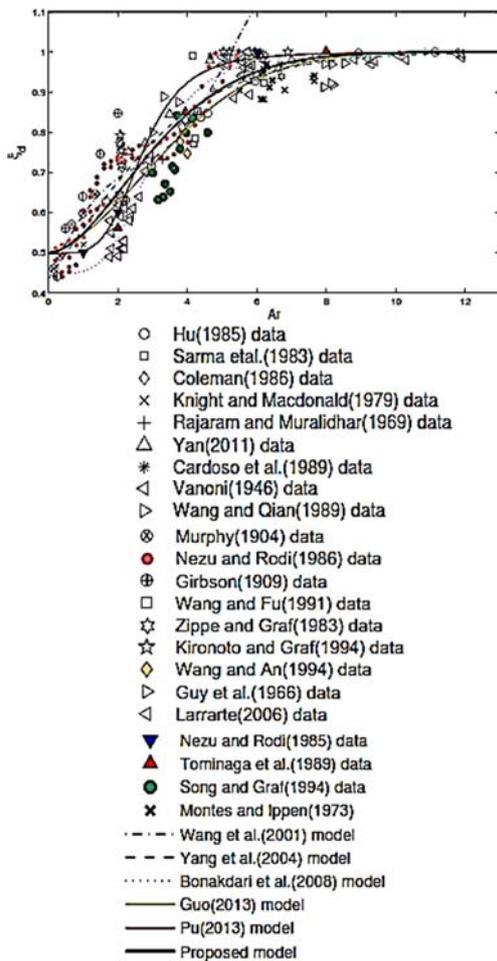
**Fig. 4. Validation of the proposed entropy model with experimental data.**
