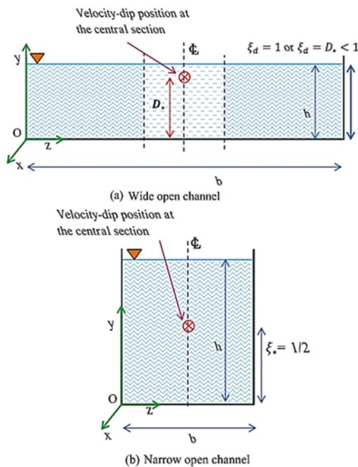
**Fig. 1. Variation of velocity-dip-position for (a) wide and (b) narrow open channels at the central section.**
