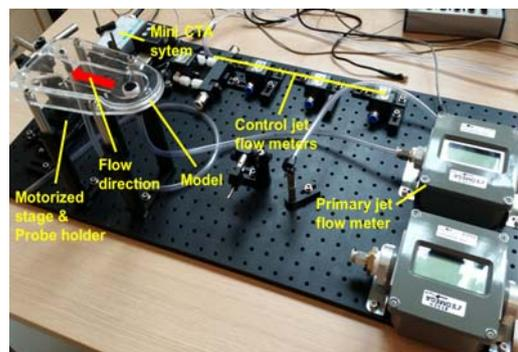
**Fig. 5. Actual experimental setup.**
