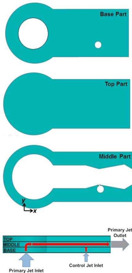
**Fig. 4. Three part design and flow paths of the primary and the control jets.**
