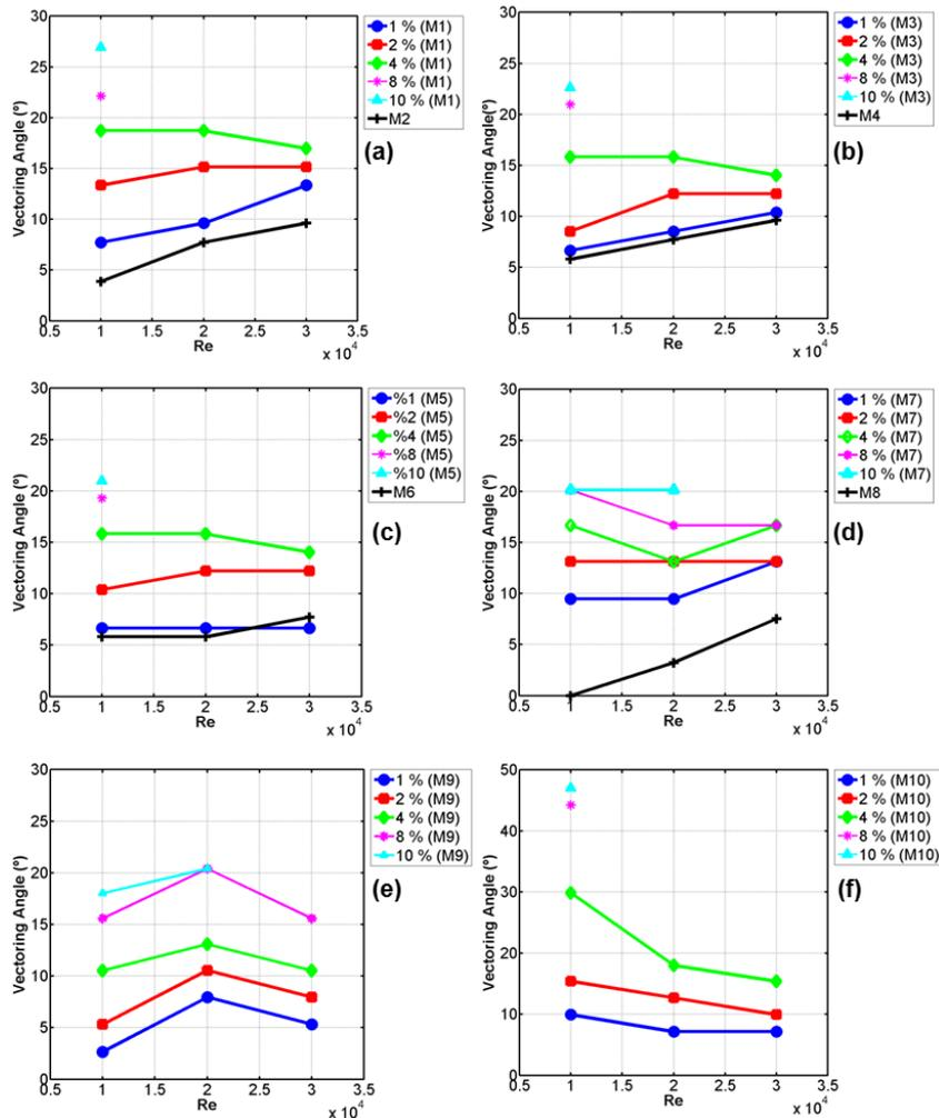
**Fig. 9.** Vectoring angles for all models for various control conditions at Re from 10000 to 30000.
