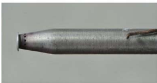
Fig. 3. Cavitator mounted on strut and the nozzles used for air injection.
