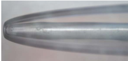
Fig. 15. Cavity formed behind parabolic type 1 cavitator.
