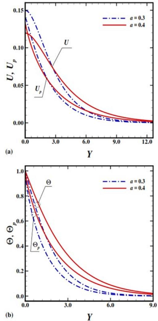
**Fig. 5. (a) Velocity and (b) Temperature profiles for  $a = 0.3, 0.4$  while  $Pr = 7.0, D_p = 10.0, \gamma = 0.1, \alpha_d = 0.1, \lambda = 1.0$  and  $X = 10.0$ .**
