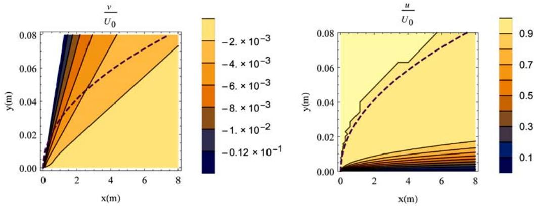
**Fig. 3. Visualization of the dimensionless vertical and mainstream velocities near the flat plate (lying in the  $xz$  plane) in the Blasius regime with  $U_0 = 0.1$  m/s and  $\nu = 10^{-6}$  m<sup>2</sup>/s.**
