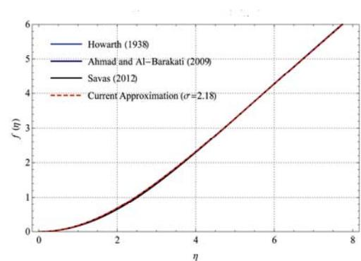
**Fig. 2. Comparison of the suggested approximation  $f''_{\sigma=2.18}(\eta)$  with the comparable schemes in Howarth (1938), Ahmad and Al-Barakati (2009) and Savas (2012). Note that the results are coincident.**
