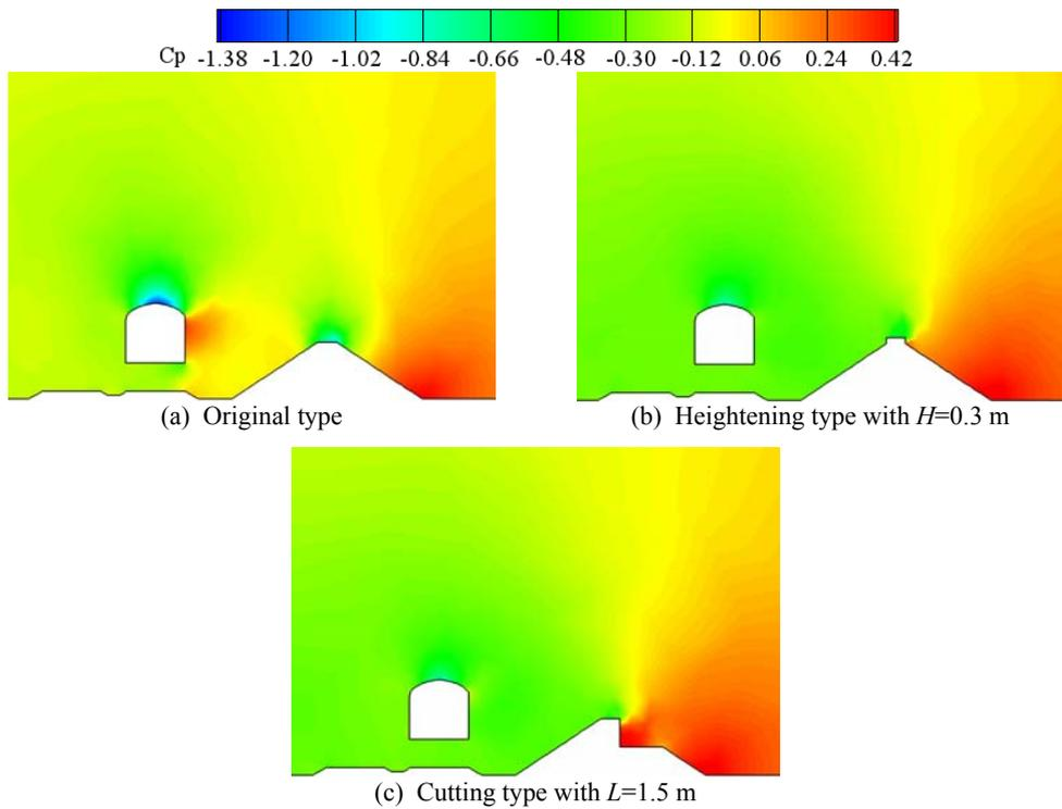
**Fig. 11. Pressure distributions around the running trains.**
