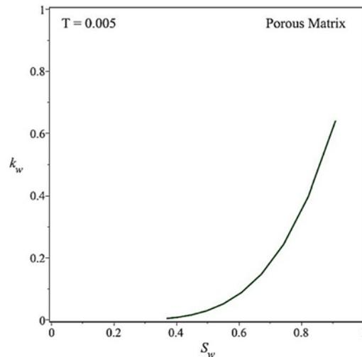
**Fig. 12. Relative permeability vs. Saturation in Porous Matrix in Fine Sand.**
