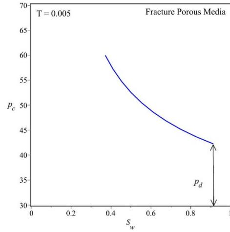
**Fig. 7. Capillary pressure vs. Saturation in Fractured Porous Media in Fine Sand.**
