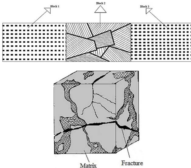
**Fig. 1. Block 1 and Block 3 are Matrix blocks and Block 2 is Fracture block.**
