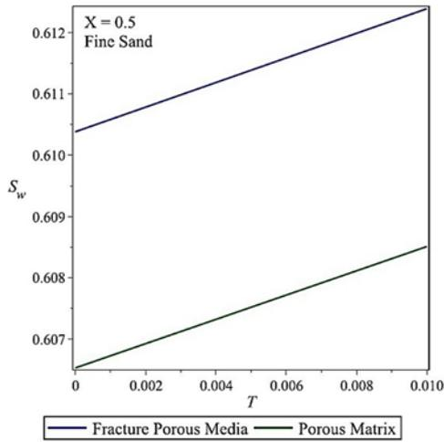
**Fig. 4. Comparison for Saturation of water vs. Dimensionless time in Fractured porous media and Porous Matrix for Fine Sand.**
