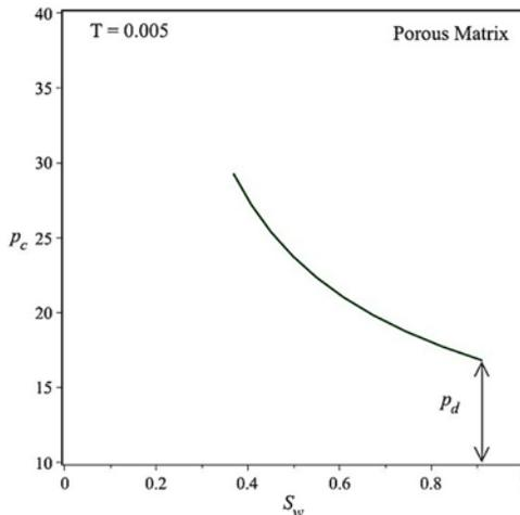
**Fig. 6. Capillary pressure vs. Saturation in Porous Matrix in Volcanic Sand.**
