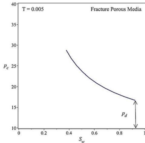
**Fig. 5. Capillary pressure vs. Saturation in Fractured Porous Media in Volcanic Sand.**
