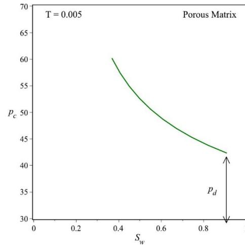
**Fig. 8. Capillary pressure vs. Saturation in Porous Matrix in Fine Sand.**
