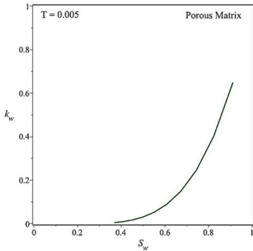
**Fig. 10. Relative permeability vs. Saturation in Porous Matrix in Volcanic Sand.**
