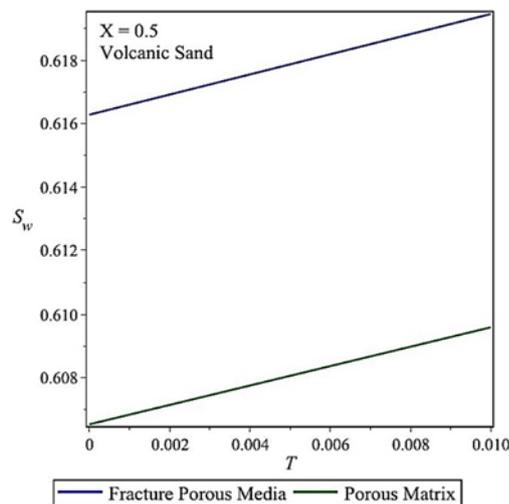
**Fig. 3. Comparison for Saturation of water vs. Dimensionless time in Fractured porous media and Porous Matrix for Volcanic Sand.**
