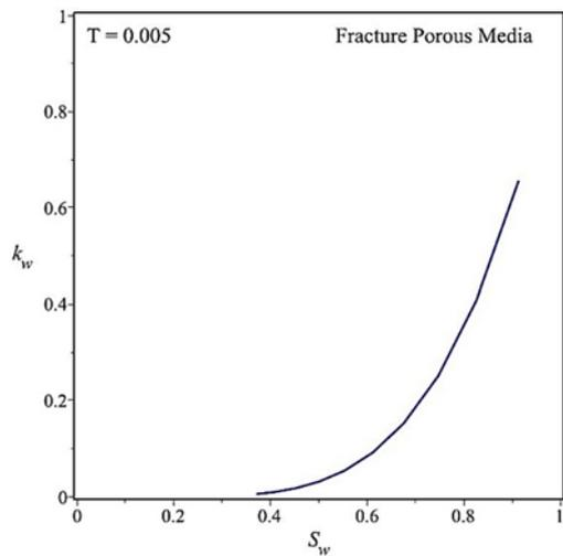
**Fig. 11. Relative permeability vs. Saturation in Fractured Porous Media in Fine Sand.**
