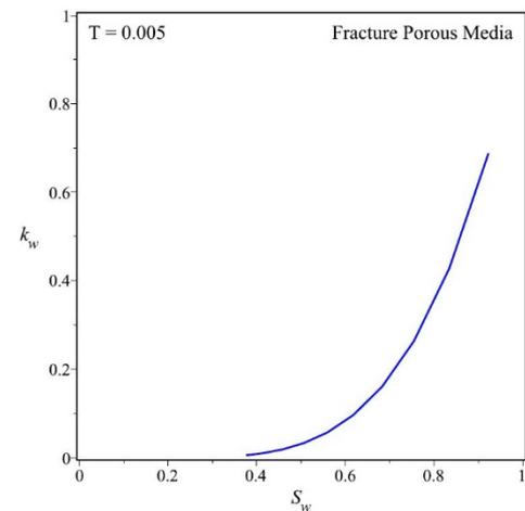
**Fig. 9. Relative permeability vs. Saturation in Fractured Porous Media in Volcanic Sand.**
