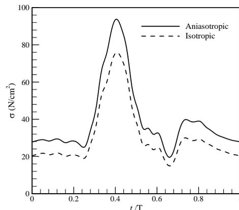
**Fig. 7. Temporal variations of the maximum wall stresses for VWT models with isotropic and anisotropic materials.**
