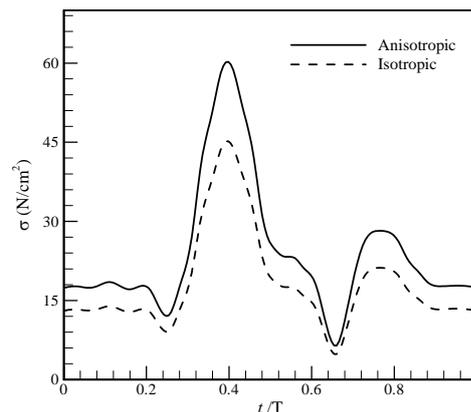
**Fig. 6. Temporal variations of the maximum wall stresses for UWT models with isotropic and anisotropic materials.**
