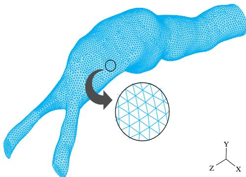
**Fig. 5. Geometrical representation of tetrahedral elements grid network in the fluid domain.**
