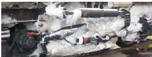
Fig. 2. Bogies covered with snow and ice.
