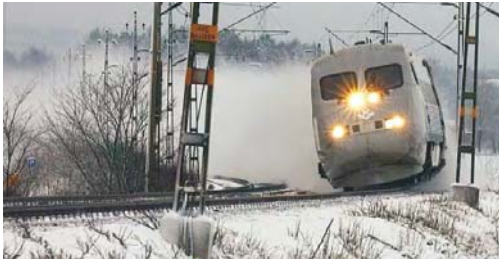
Fig. 1. Snow smoke produced by the tilting train of the Swedish X2.
