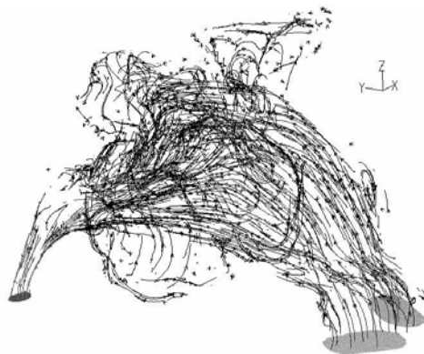
Fig. 5. Airflow streamlines for breathing speed of 1.111 m/s.
