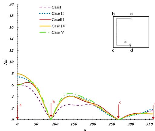
**Fig. 10. Comparison of local Nusselt number of outer cavity in Ra=10<sup>5</sup>, ε=0.4, and Darcy number of 0.01.**
