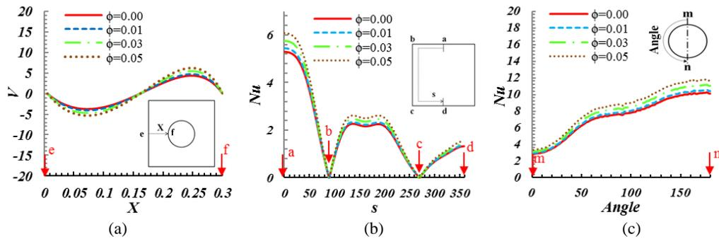
**Fig. 8.** Effect of nanoparticle volume fraction on (a) velocity profile, (b) local Nusselt number of the outer wall and (c) local Nusselt number of the inner cylinder,  $Ra=10^5$   $\epsilon=0.4$  and  $Da=0.01$  (Case I).
