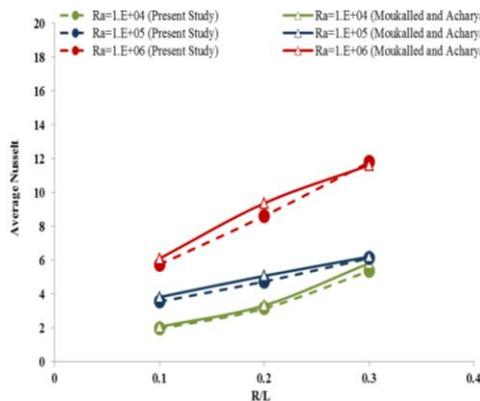
**Fig. 6. Comparison of the average Nusselt number between the present study and the numerical results by [Moukalled and Acharya \(1996\)](#).**
