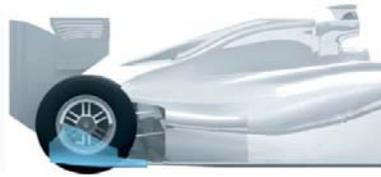
Fig. 1. Diffuser region under a sample car.
