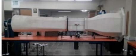
Fig. 5. Open loop wind tunnel.
