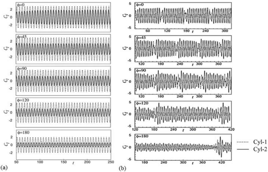
**Fig. 8. Time series of lift coefficient with change in  $\phi$  for  $f_r = 1.2$ , (a)  $S = 2D$  (b)  $S = 5D$**
