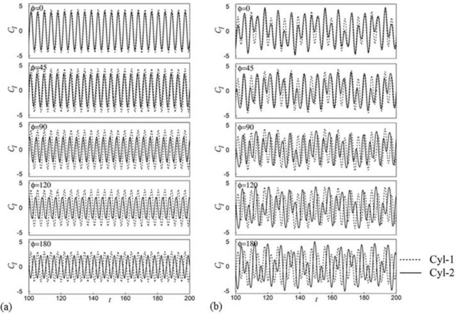
**Fig. 9. Time series of lift coefficient with change in  $\phi$  for  $f_r = 1.6$ , (a)  $S = 2D$  (b)  $S = 5D$**
