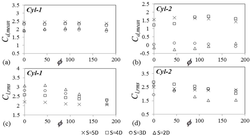
**Fig. 17. Variation of lift and drag coefficients with phase difference for different  $S$  at  $f_r = 1.6$**
