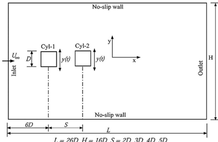
**Fig. 1. Schematic of computational domain**
