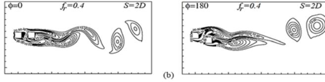
**Fig. 10. Vorticity contours with change in  $\phi$  at sub - synchronous frequency**
