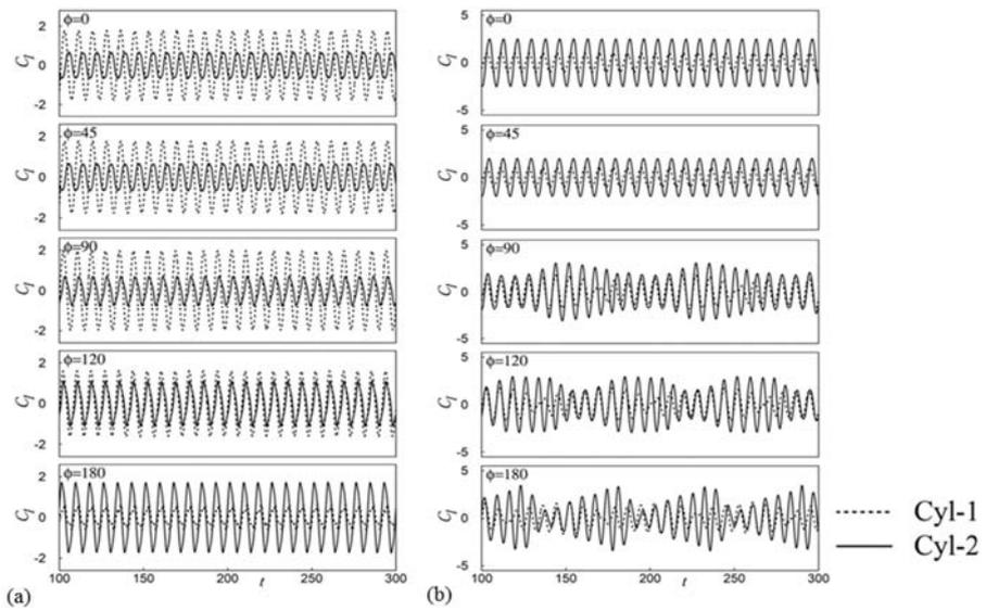
Fig. 6. Time series of lift coefficient with the change in  $\phi$  for  $f_r = 0.8$ , (a)  $S = 2D$  (b)  $S = 5D$
