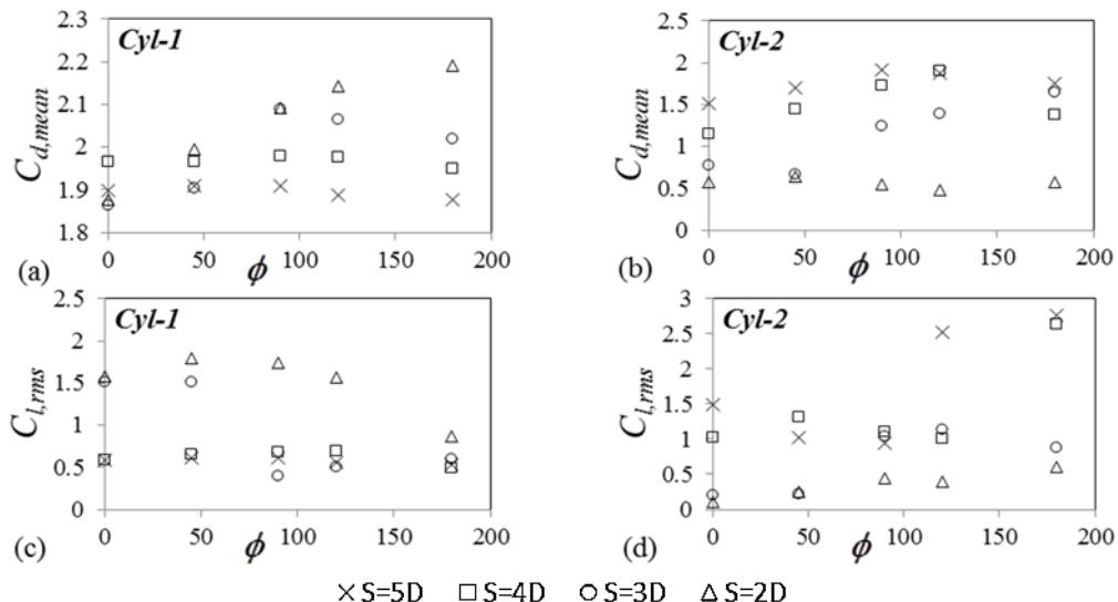
Fig. 15. Variation of lift and drag coefficients with phase difference for different  $S$  at  $f_r = 1$
