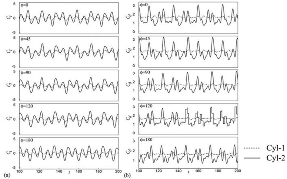
**Fig. 4.** Time series of lift and drag with the change in  $\phi$  for  $f_r = 0.4$  and  $S = 5D$
