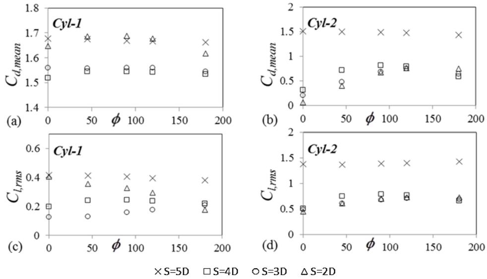
Fig. 13. Variation of lift and drag coefficients with phase difference for different  $S$  at  $f_r = 0.4$
