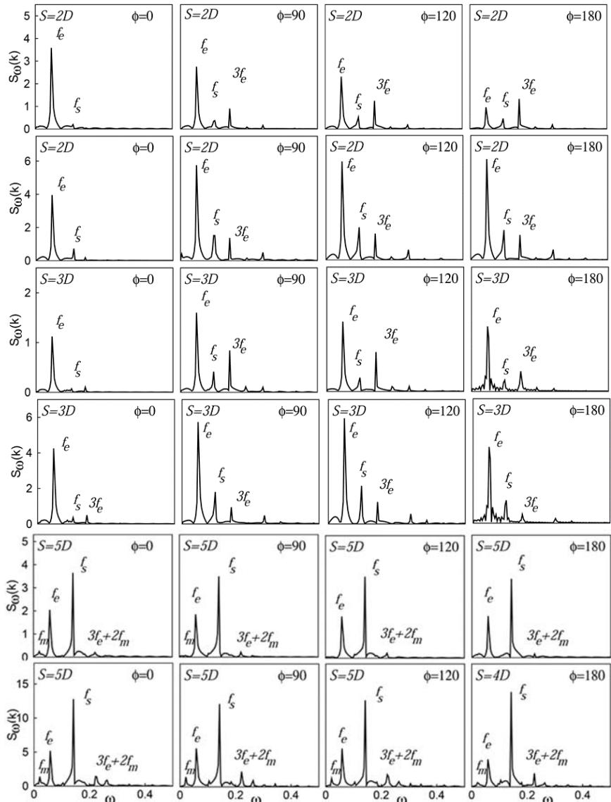
**Fig. 5. Fourier spectra of lift signal for the upstream (upper row) and downstream cylinders (lower row) at  $f_r = 0.4$  with change in phase for  $S = 2D, 3D$  and  $5D$**
