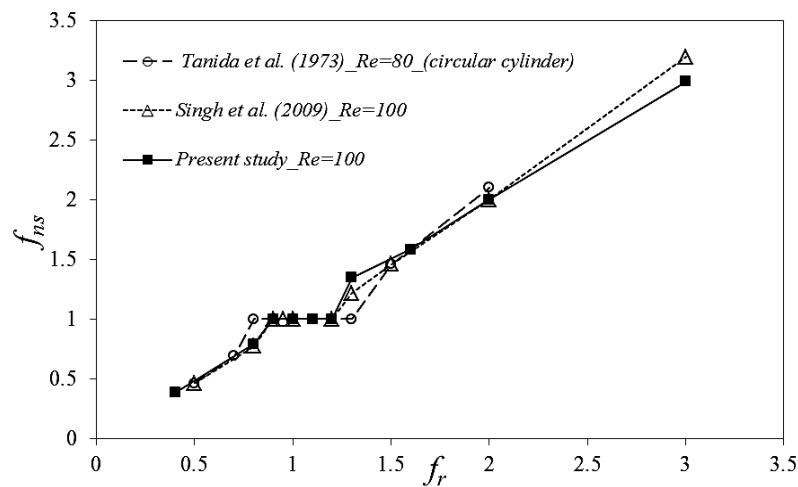
**Fig. 2. Comparison of lock-in band of frequency for single cylinder oscillation (Mithun and Tiwari, 2014)**
