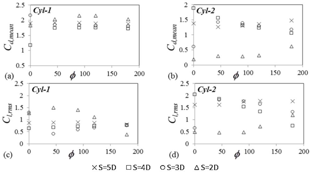
Fig. 14. Variation of lift and drag coefficients with phase difference for different  $S$  at  $f_r = 0.8$
