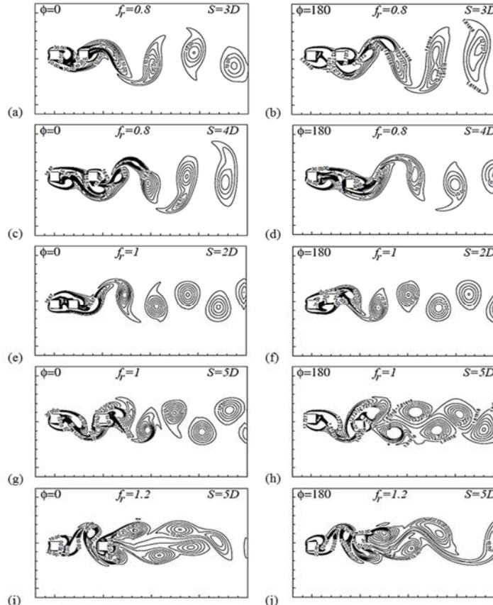
**Fig. 11. Vorticity contours showing variation in shedding pattern with change in  $\phi$  for selected spacing at synchronous frequencies**
