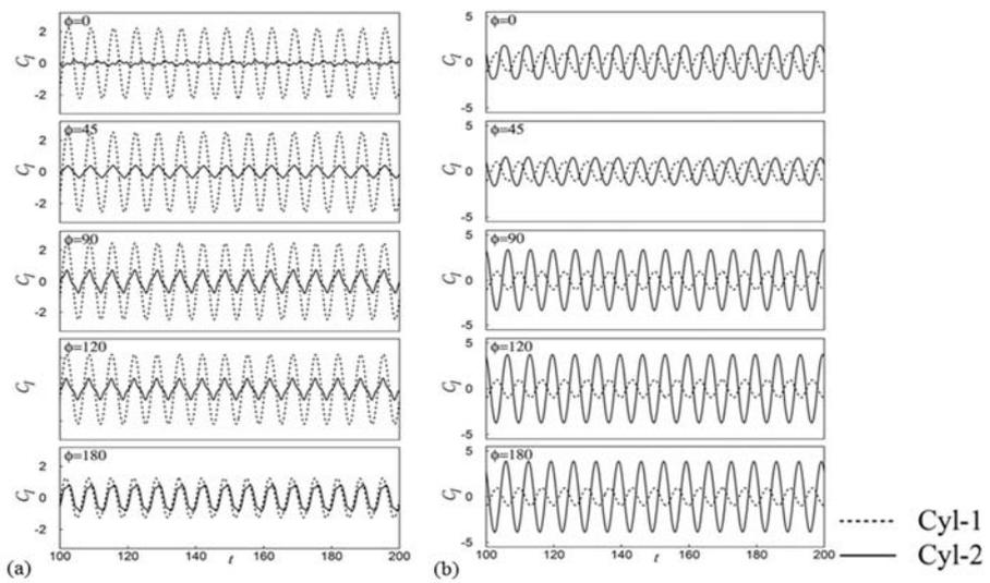
Fig. 7. Time series of lift coefficient with the change in  $\phi$  for  $f_r = 1$ , (a)  $S = 2D$  (b)  $S = 5D$
