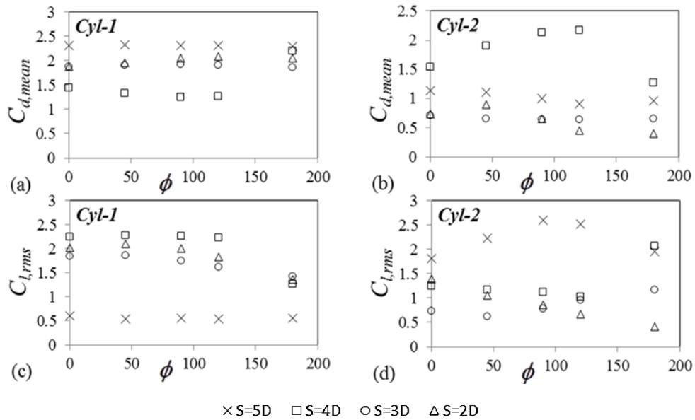
**Fig. 16. Variation of lift and drag coefficients with phase difference for different  $S$  at  $f_r = 1.2$**
