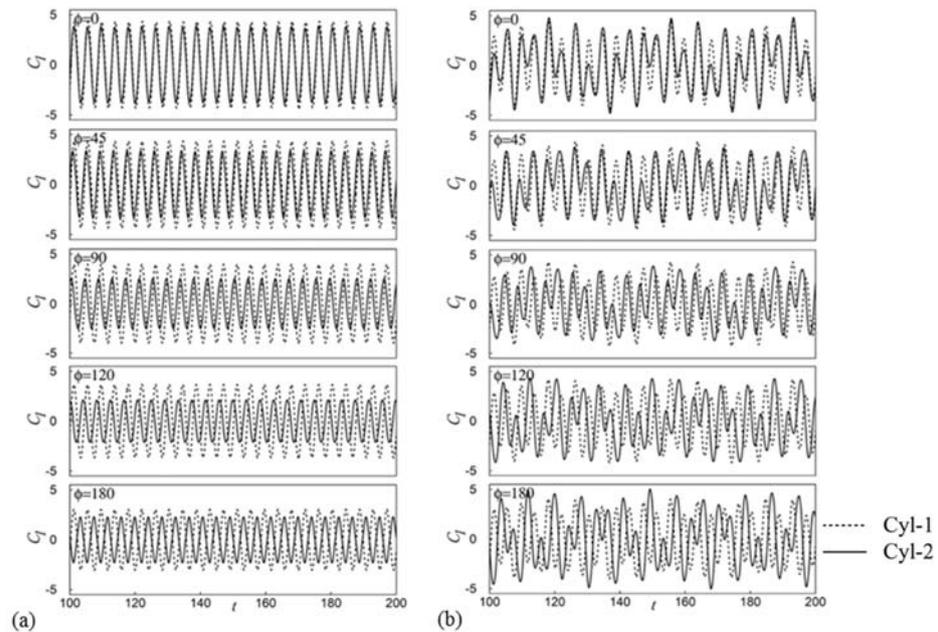
**Fig. 9. Time series of lift coefficient with change in  $\phi$  for  $f_r = 1.6$ , (a)  $S = 2D$  (b)  $S = 5D$**
