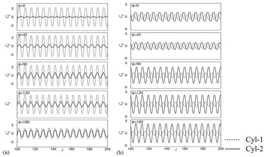
**Fig. 7. Time series of lift coefficient with the change in  $\phi$  for  $f_r = 1$ , (a)  $S = 2D$  (b)  $S = 5D$**
