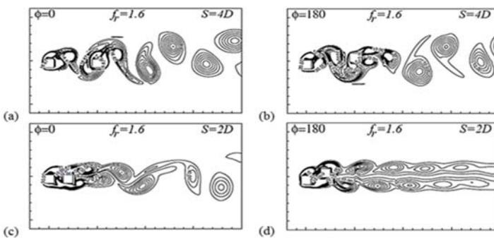
**Fig. 12. Vorticity contours showing variation in shedding pattern with change in  $\phi$  for selected spacing at super - synchronous frequency**
