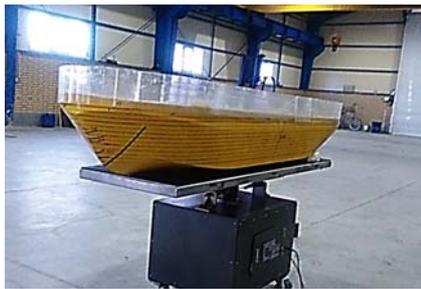
Fig. 6. Measuring moment of inertia using the oscillating table.
