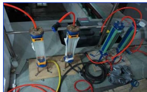
**Fig. 3. Glass rotor flow meter**
