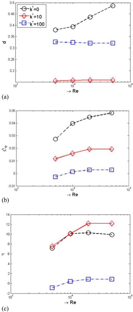
**Fig. 17. Variation of overall extent of vertical displacement ( $d$ ), net coefficient of power ( $\bar{C}_{op}$ ) and power extraction efficiency ( $\eta$ ) with changing Reynolds numbers ( $Re$ ). Semi-passive flapping NACA0015 airfoil at  $f^*=0.1$ ,  $b^*=2\pi$ ,  $\theta_0=15^\circ$ .**
