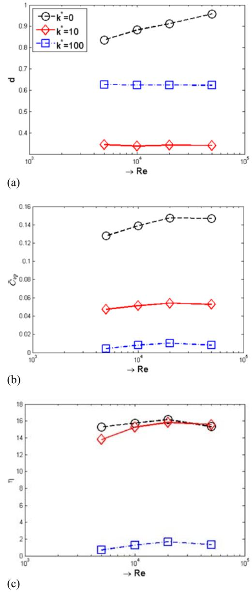
**Fig. 18. Variation of overall extent of vertical displacement ( $d$ ), net coefficient of power ( $\bar{C}_{op}$ ) and power extraction efficiency ( $\eta$ ) with changing Reynolds numbers ( $Re$ ). Semi-passive flapping NACA0015 airfoil at  $f^*=0.1$ ,  $b^*=2\pi$ ,  $\theta_0=30^\circ$ .**
