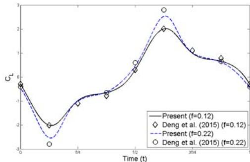
**Fig. 8. Time-dependent variation of vertical force coefficient ( $C_y$ ) for pitch-activated flapping NACA0015 airfoil during single oscillation period at  $Re=1000$ ,  $\theta_0=75^\circ$ ,  $k^*=0$ ,  $b^*=\pi$ ,  $m^*=0.1022$ . Results compared with the solutions obtained by Deng et al. (2015).**
