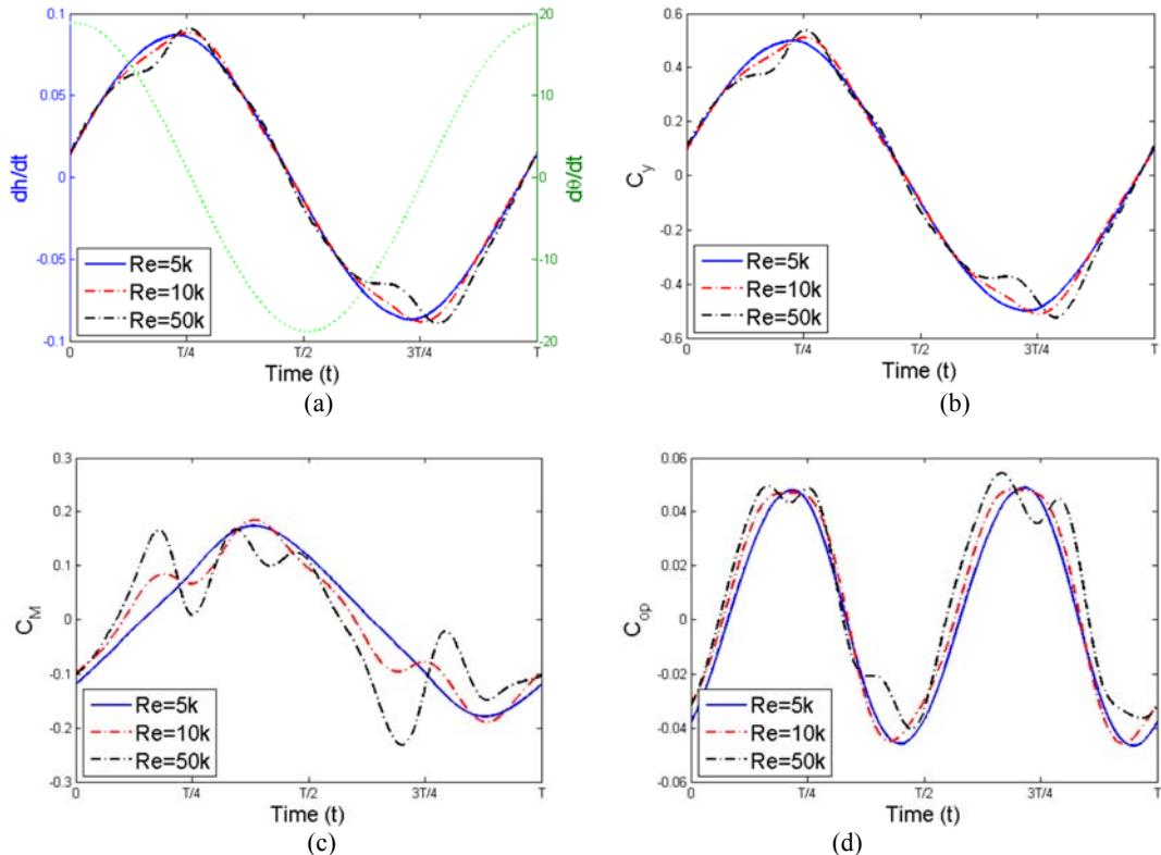
**Fig. 9.** Profiles of heave and pitch velocities ( $dh/dt$  and  $d\theta/dt$ ), vertical force and moment coefficients ( $C_y$ ,  $C_M$ ) and coefficient of power ( $C_{op}$ ) during a single oscillation period and at different Reynolds number for semi-passive flapping NACA0015 airfoil at  $f^* = 0.2$ ,  $k^* = 0$ ,  $b^* = 2\pi$  and  $\theta_0 = 15^\circ$ .
