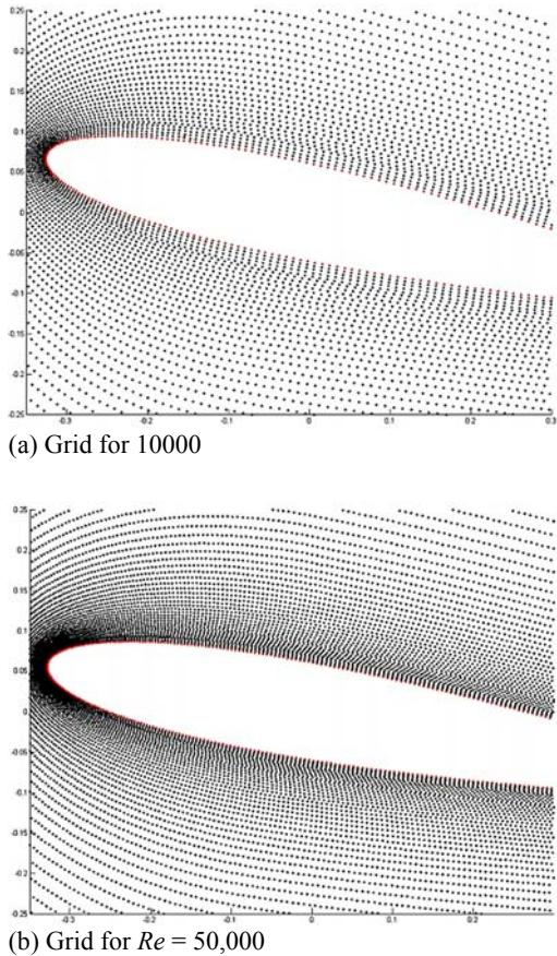
**Fig. 6. Modeled grid for multiple Reynolds numbers around NACA0012 airfoil.**
