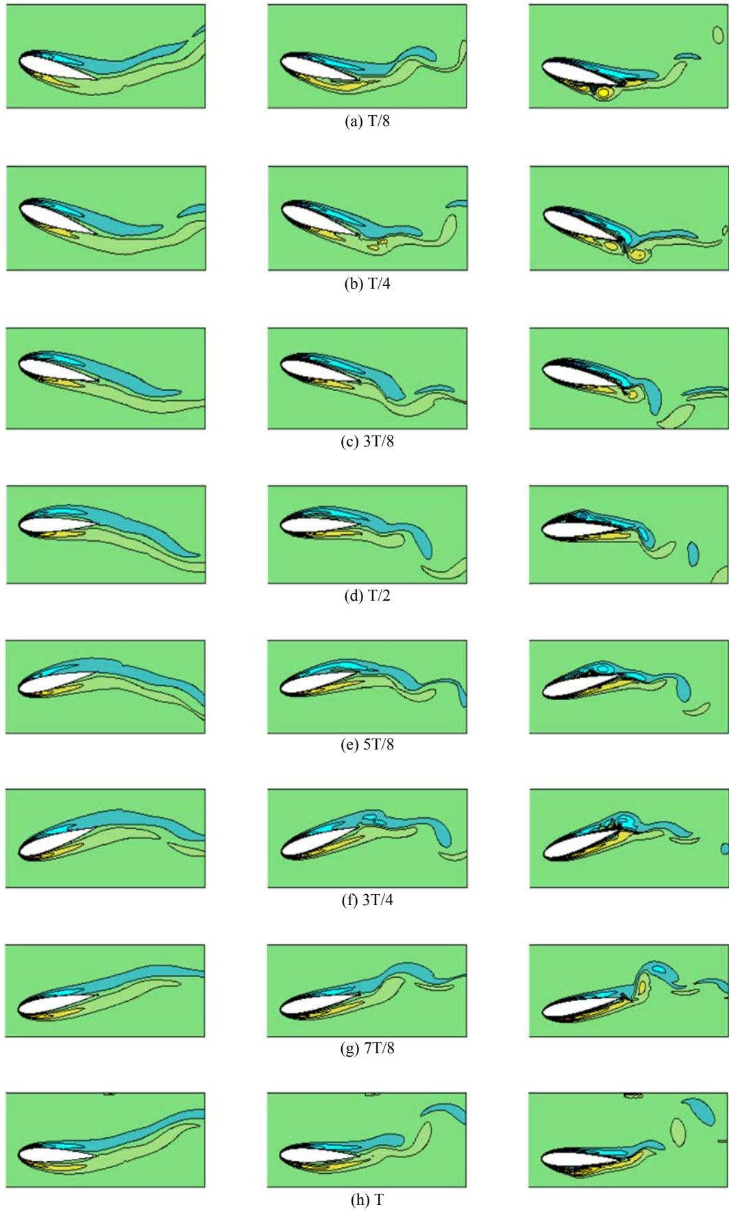
Fig. 11. Instantaneous vorticity profiles around pitch-activated flapping airfoil (NACA0015 at  $k^*=0$ ,  $b^*=2\pi$ ,  $\theta_0=15^\circ$ ,  $f^*=0.2$ ). Lt column:  $Re=5000$ , center column:  $Re=10000$ , Rt column:  $Re=50000$ .
