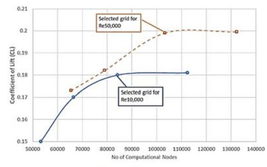
**Fig. 5. Grid independence check carried out at  $Re=10,000$  and  $Re=50,000$  at  $AoA = 5 \text{ deg}$  for NACA0012.**
