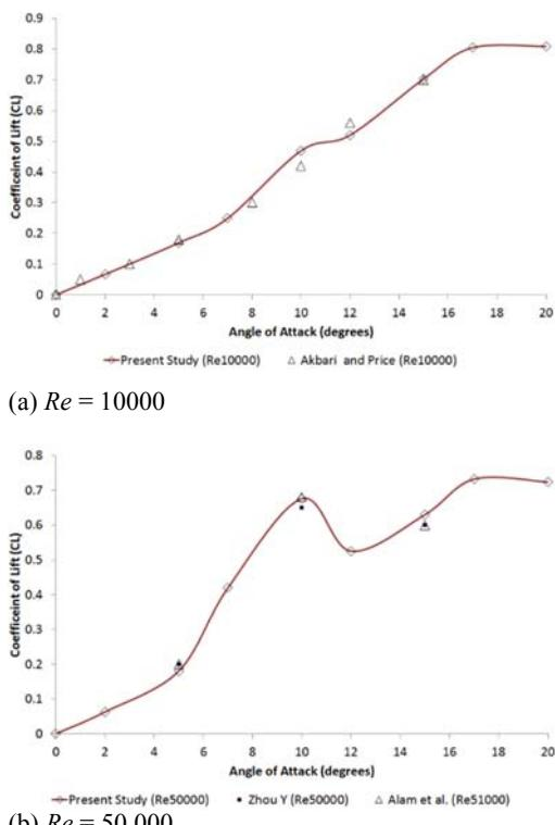
**Fig. 7.  $C_L$  vs  $\alpha$  curves for multiple Reynolds number around NACA0012 airfoil.**
