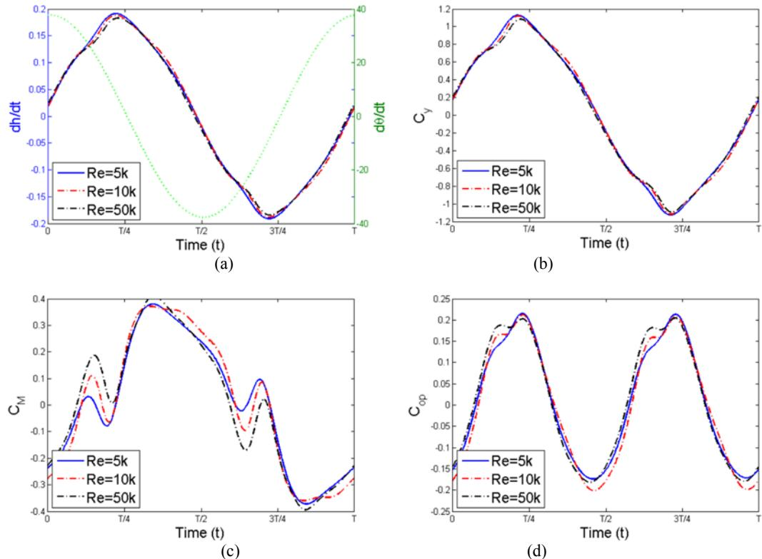
**Fig. 10.** Profiles of heave and pitch velocities ( $dh/dt$  and  $d\theta/dt$ ), vertical force and moment coefficients ( $C_y$ ,  $C_M$ ) and coefficient of power ( $C_{op}$ ) during a single oscillation period and at different Reynolds number for semi-passive flapping NACA0015 airfoil at  $f^* = 0.2$ ,  $k^* = 0$ ,  $b^* = 2\pi$  and  $\theta_0 = 30^\circ$ .
