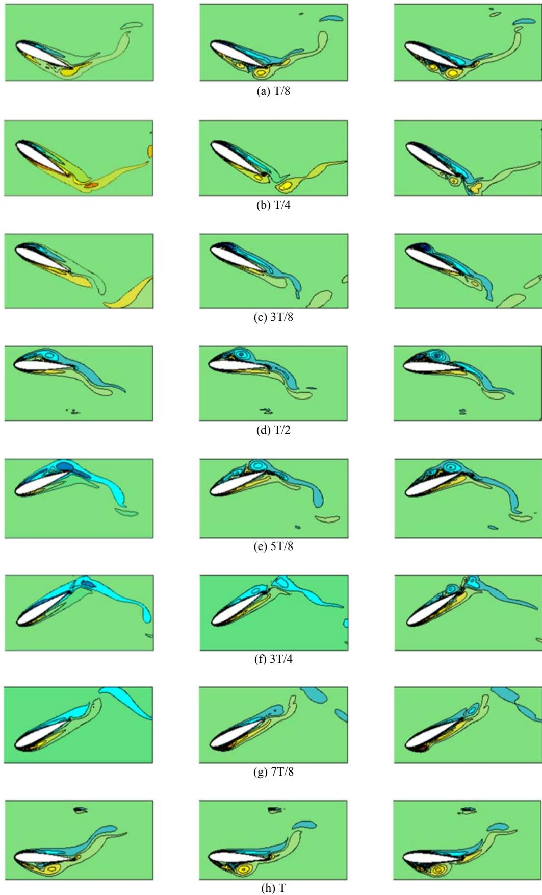
**Fig. 12. Instantaneous vorticity profiles around pitch-activated flapping airfoil (NACA0015 at  $k=0$ ,  $b=2\pi$ ,  $\theta_0=30^\circ$ ,  $f=0.2$ ). Lt column:  $Re=5000$ , center column:  $Re=10000$ , Rt column:  $Re=50000$ .**
