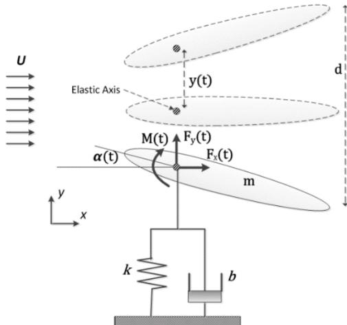
**Fig. 1. Schematic of Pitching motion activated flapping foil.**
