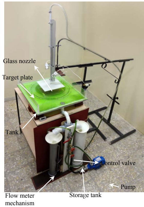
Fig. 2. Experimental apparatus for creating the circular hydraulic jumps
