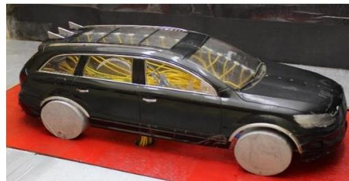
**Fig. 1.3** Car model with right angle design VGs.
