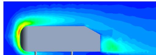
**Fig. 2.4 Turbulent kinetic energy of base Ahmed body.**
